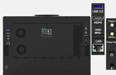
Standard with BNC adapter. Equipped with abundant ports including USB 3.0/2.0 Host, USB Type-C, LAN, HDMI, Aux In/Out and 10MHz clock signal In/Out.
