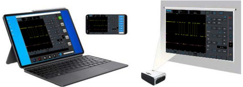
MHO 6 series support PC and smartphone remote control, also have HDMI port for demonstration purpose. Support SCPI programming commands control, helping engineers achieve automated measurements more flexibly and efficiently.
