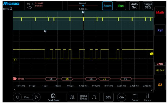
**Serial bus decoding and analysis**
