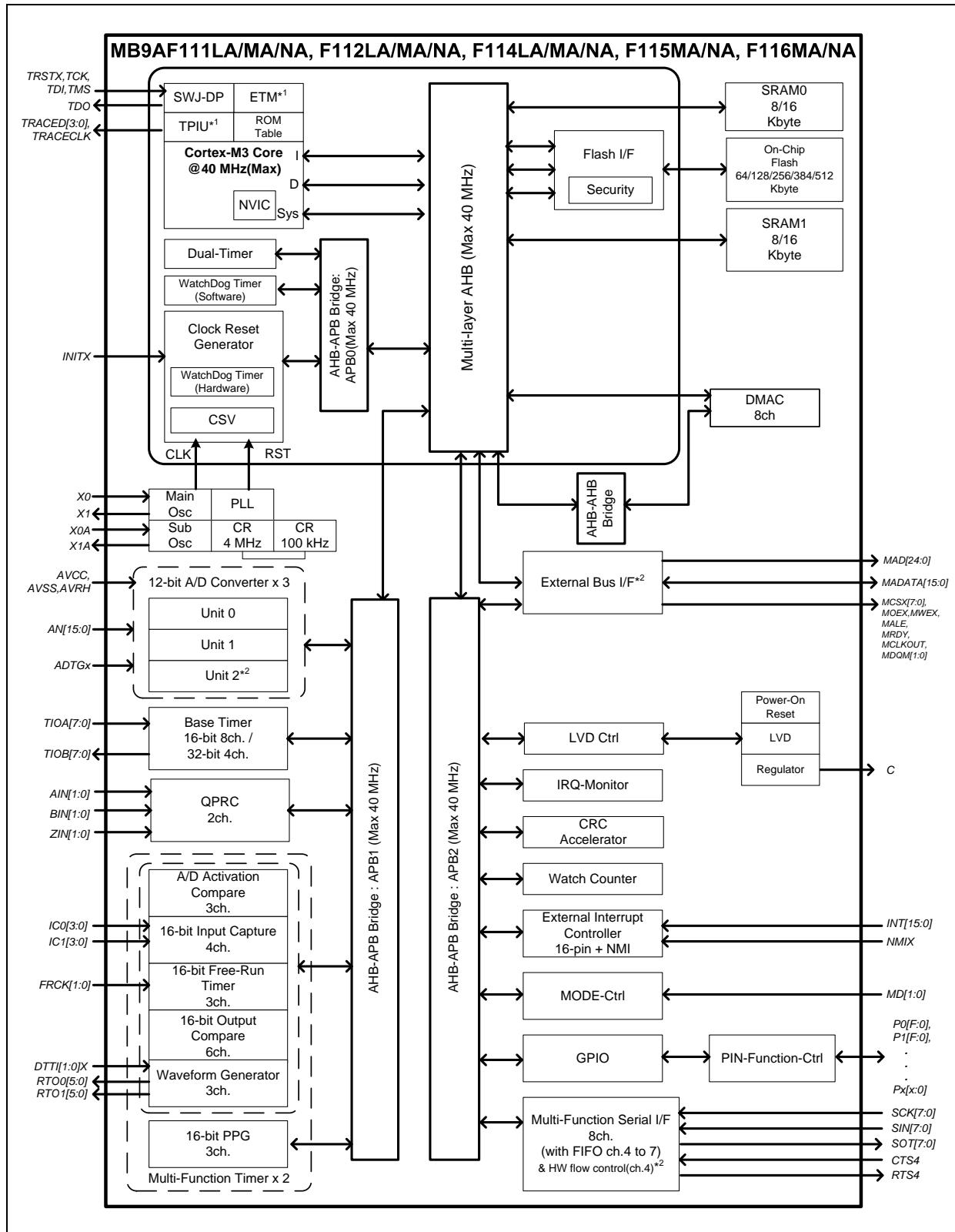
\*1: For the MB9AF111LA/MA, F112LA/MA, MB9AF114LA/MA, MB9AF115MA and MB9AF116MA, ETM is not available.
