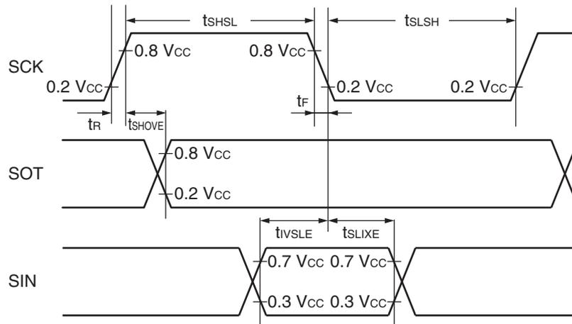
Sampling is executed at the rising edge of the sampling clock\*1, and serial clock delay is enabled\*2.
