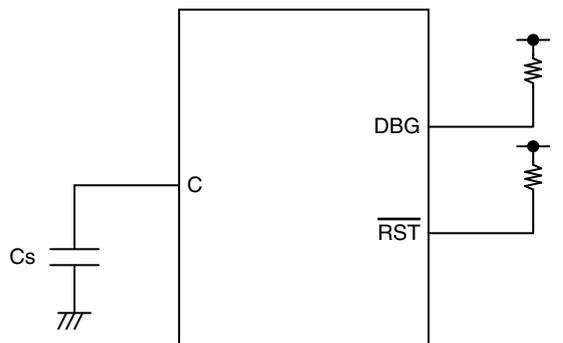
\*: Since the DBG pin becomes a communication pin in on-chip debug mode, set a pull-up resistor value suiting the input/output specifications of P12/DBG/EC0.
