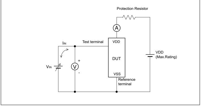
Note : The voltage V<sub>IN</sub> is increased gradually and the current I<sub>IN</sub> of 300 mA at maximum shall flow. Confirm the latch up does not occur under I<sub>IN</sub> = ± 300 mA.
