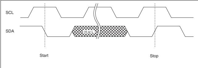
Note : At the write operation, the FeRAM device does not need the programming wait time (twc) after issuing the Stop Condition.
