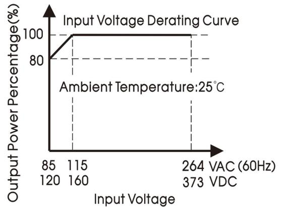
Note: ① With an input voltage between 85 -115VAC and a DC input between 120-160VDC the output power must be derated as per the temperature derating curves;
