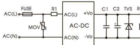
Fig 2: EMC application circuit with higher requirements
