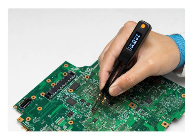
LCR Elite1 is a digital multimeter designed to measure inductance, capacitance and resistance with high accuracy. It is small, light and super-convenient for you to carry everywhere and not be tethered to bulky lab equipment.
