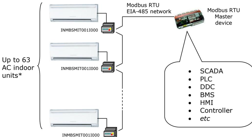
\* Up to 63 Intesis devices can be installed in the same Modbus RTU bus. However, the installation of Modbus Repeaters may be required.
