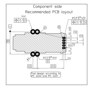
2.15 mm for primary pin 0.9 mm for secondary pin
