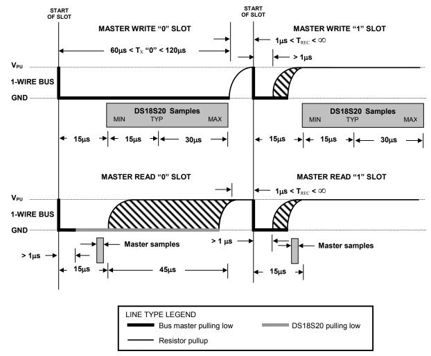
READ/WRITE TIME SLOT TIMING DIAGRAM Figure 11
