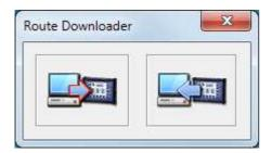
Press button (used for uploading to the instrument) select your rdi or rvi file and press Open. The route will be uploaded into the instrument.
