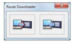
Press button (used for downloading from the instrument). The Route Downloader creates rdx or rvx file which is readable for DDS software. Choose the rdx/rvx file location, name it and save.
