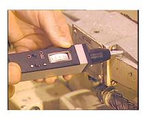
The UL101 Receiver shown here with 1-inch solid probe testing solenoid valves for bypass leak Originally designed for the US Military, the CTRL UL101 Ultrasound Inspection Kit is now used in numerous industries throughout the world for predictive maintenance, quality control, and leak detection.
