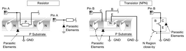
Example of Monolithic IC Structure
