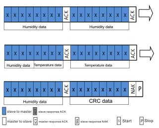
Note: The sensor needs time to collect, after the host sendsout the measurement command (0xAC), delay for more than80 ms to read the converted data and judge whether the returned status bit is normal or not.If the status bit [Bit7] is 0, the data can be read normally, 1, the sensor is busy, the host needs to wait for the completion of data processing.
