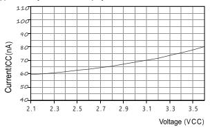
Figure 7: At a temperature of  $25^{\circ}$ C, the typical supply current is plotted against the supply voltage (sleep mode). Note that the deviation from the displayed value may be  $\pm 50\%$  of the displayed value. At  $60^{\circ}$ C, the coefficient is approximately 15 (compared with Table 2)
