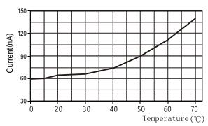
Figure 6: When VCC=3.3V, the relationship curve between typical supply current and temperature (sleep mode).Note that these data are approximately ±25% off the displayed values.
