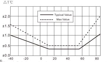
Figure 3 Typical error and maximum error temperature Temperature (°C)
