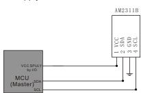
Figure 8-1 Typical Application Circuit 1, the SDA pull-up voltage and VCC are supplied by the MCU.
