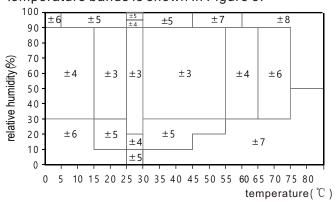
Figure 5 :The maximum error of humidity in the range of  $0\sim80(^{\circ}C)$ , unit: (%RH)
