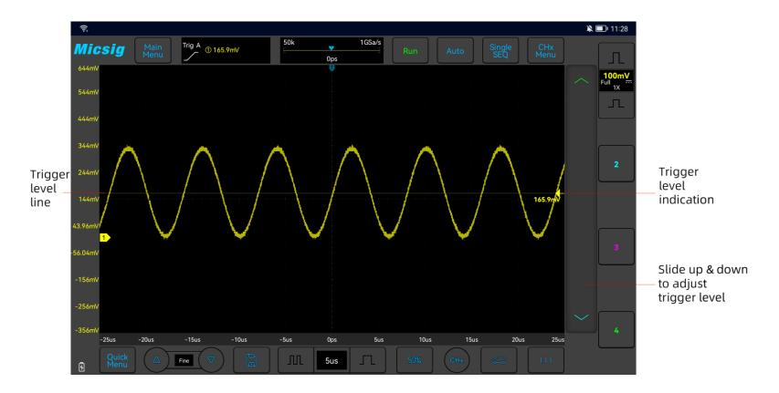
Figure 6-8 Trigger Level
