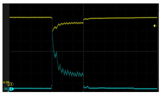
Figure 3-7 Starting voltage and current
