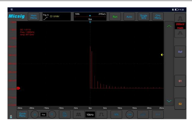
Figure 9-4 Spectrum Amplitude as V-Hz
