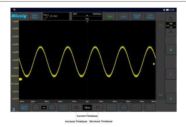
Figure 4-3 Adjust the Horizontal Time Base
