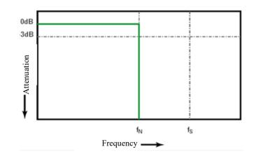
Figure 11-2 Theoretical Brick-Wall Frequency Response
