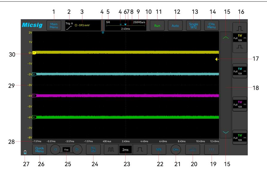
Figure 2-6 Oscilloscope Interface Display
