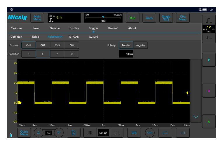
Figure 6-13 Pulse Width Trigger Setting Menu
