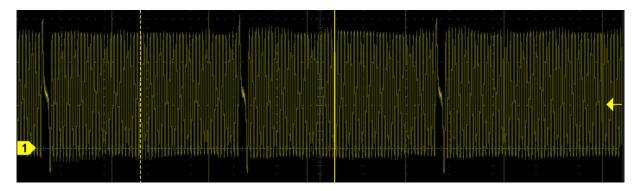
Figure 3-18 Actual measurement diagram of crankshaft position sensor (inductive type)
