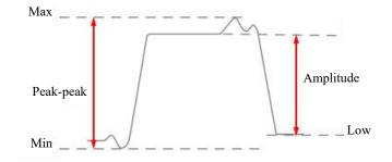
Figure 7-5 Voltage Measurement
