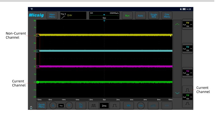
Figure 5-2 Current Channel and Non-Current Channel
