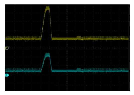
Figure 3-12 Actual measured waveform of accelerator pedal sensor
