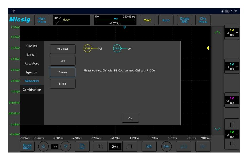
Figure 3-53: FlexRay bus test
