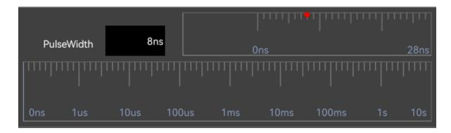
Figure 6-19 Pulse Width Time Adjustment Interface
