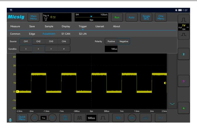
Figure 6-14 Negative Polarity Pulse Level Flip
