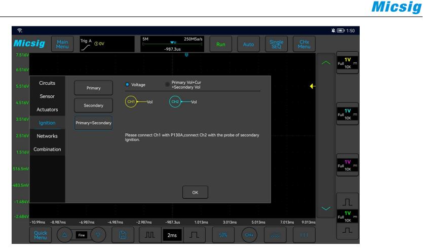
Figure 3-47: Primary + Scondary ignition test
