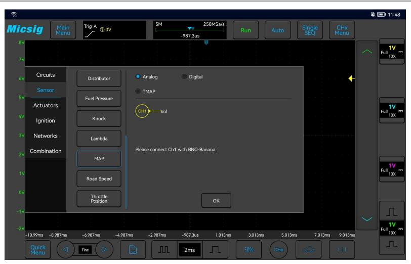
Figure 3-25 MAP (intake pressure sensor)
