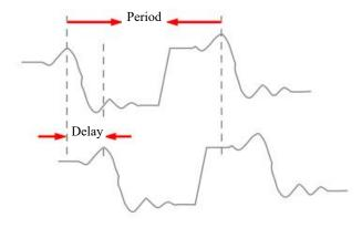
Figure 7-4 Phase Measurement Schematics
