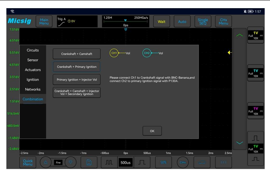
Figure 3-56 Crankshaft + Primary ignition test
