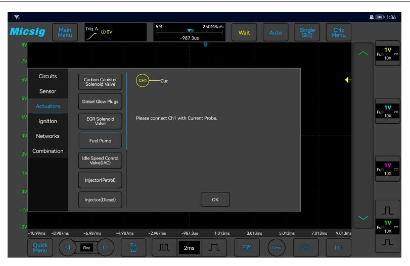
Figure 3-33 Electronic fuel pump test
