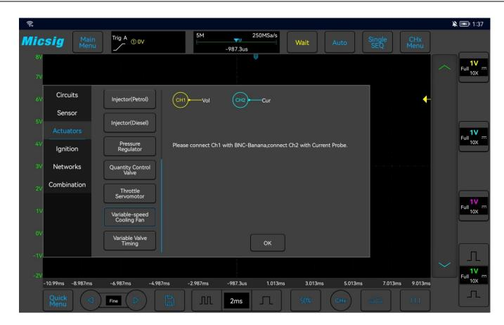
Figure 3-40 Variable-speed Cooling fan test
