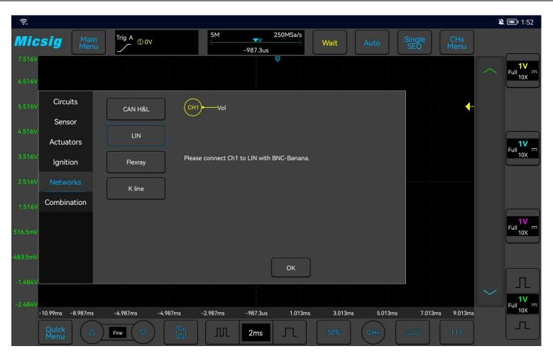
Figure 3-51 Lin bus test
