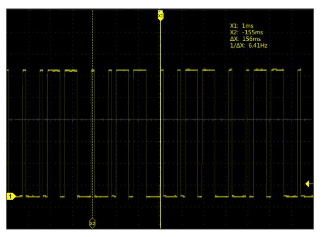
Figure 3-15 Camshaft position sensor (Hall type)
