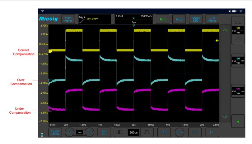
Figure 2-11 Probe Compensation
