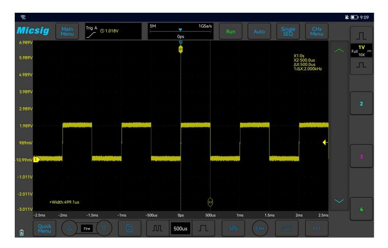
Figure 7-8 Cursor Measurement Pulse Width
