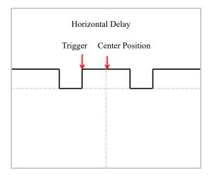
Figure 6-7 Horizontal Delay
