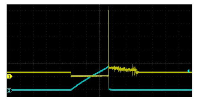
Figure 3-48 BMW 5 Series N20 Primary + Secondary ignition signal
