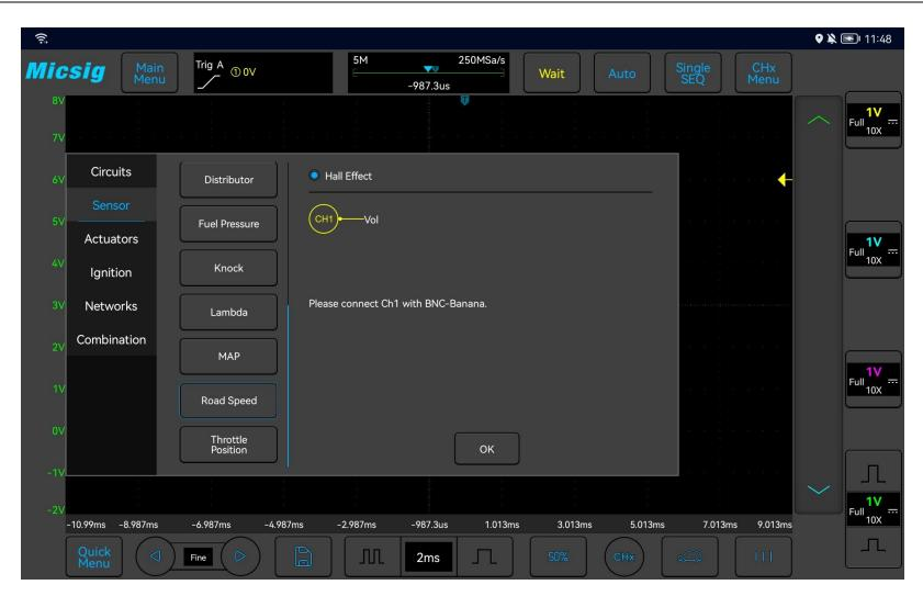
Figure 3-26 Vehicle speed sensor test
