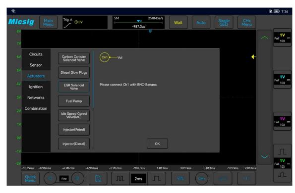
Figure 3-32 EGR solenoid valve test
