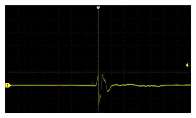
Figure 3-22 Actual measurement chart of knock sensor
