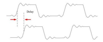
Figure 7-3 Delay Measurement Schematics
