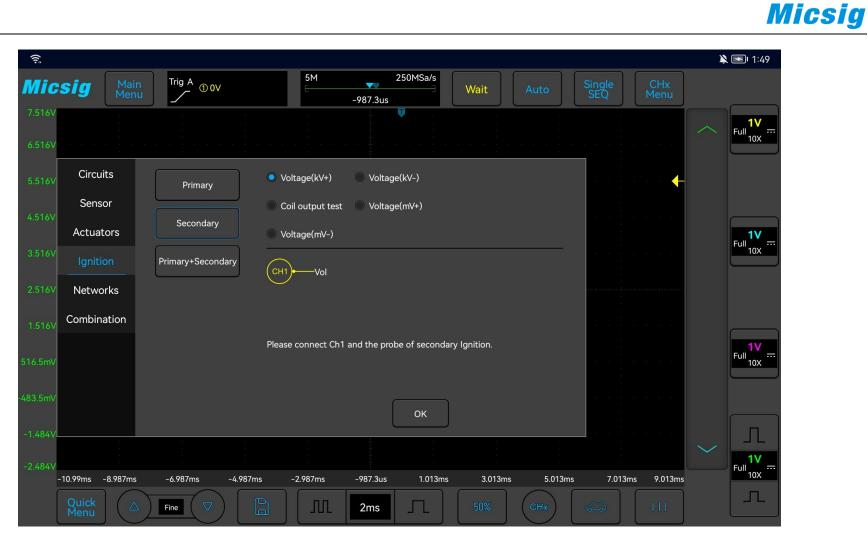
Figure 3-46 Secondary ignition test
