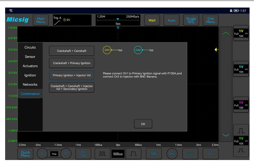
Figure 3-57 Primary ignition + Injector voltage
