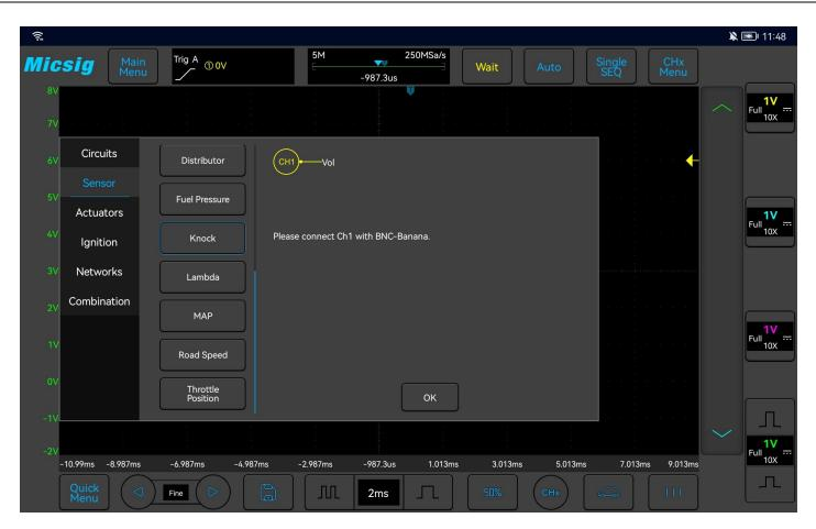
Figure 3-21 Knock Sensor test
