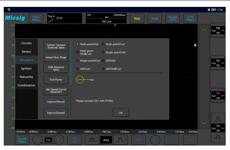
Figure 3-35 Injector (Petrol) Test
