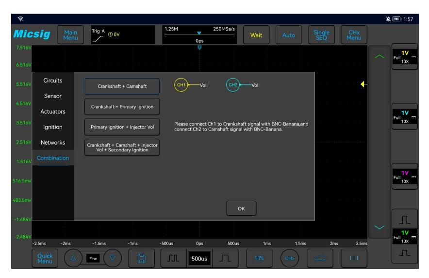
Figure 3-55 Crankshaft + Camshaft Combination Test
