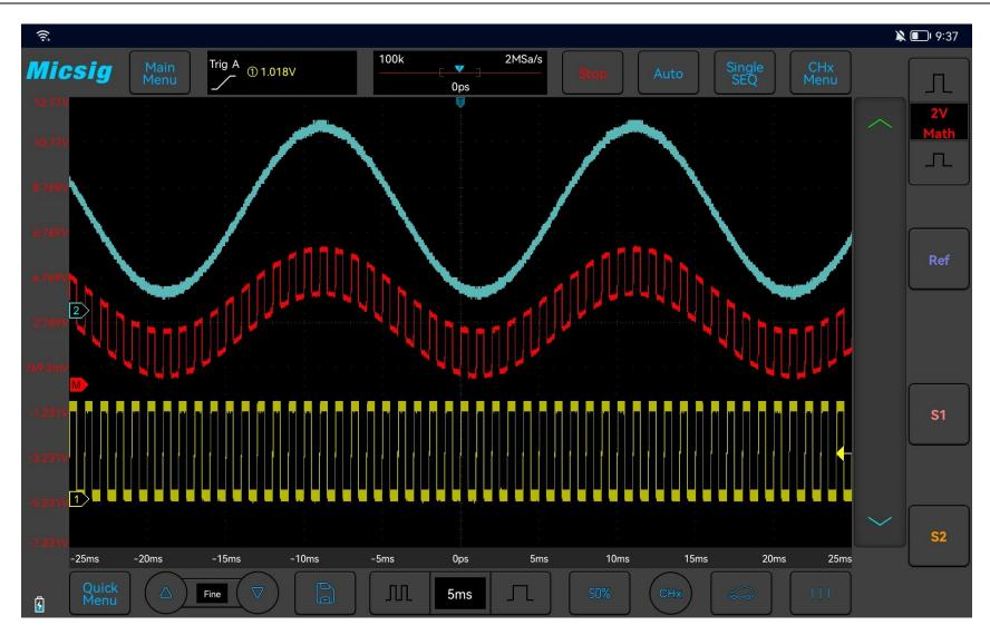
Figure 9-2 Mathematical Operation of CH1 adding CH2
