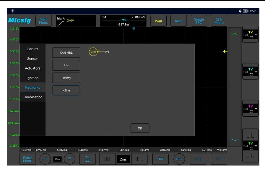
Figure 3-54 K line test
