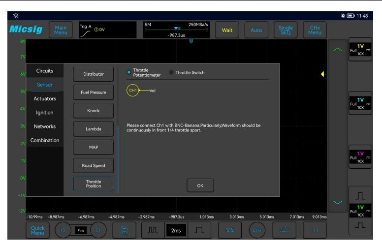
Figure 3-27 Throttle Position Sensor test
