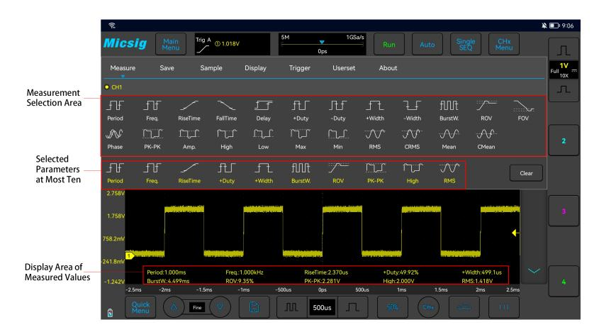
Figure 7-1 Automatic Measurement Menu
