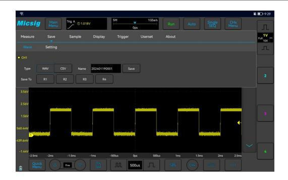
Figure 8-1 Save CH1 Reference Waveform Interface
