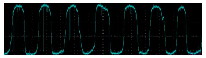
Figure 3-24 Lambda (Oxygen Sensor) diagram
