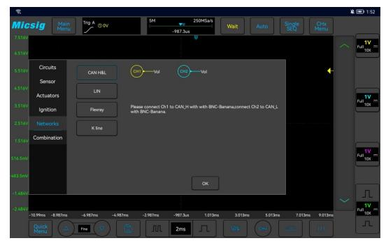
Figure 3-49 CAN BUS Test
