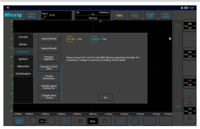
Figure 3-39 Throttle servo motor test
