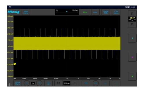
Figure 6-3 Abnormal Signal in Periodic Signals
