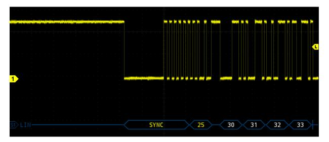
Figure 3-52 Audi A6 LIN bus measurement
