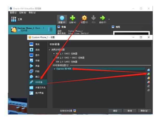
Figure 2-4 Setting USB device
