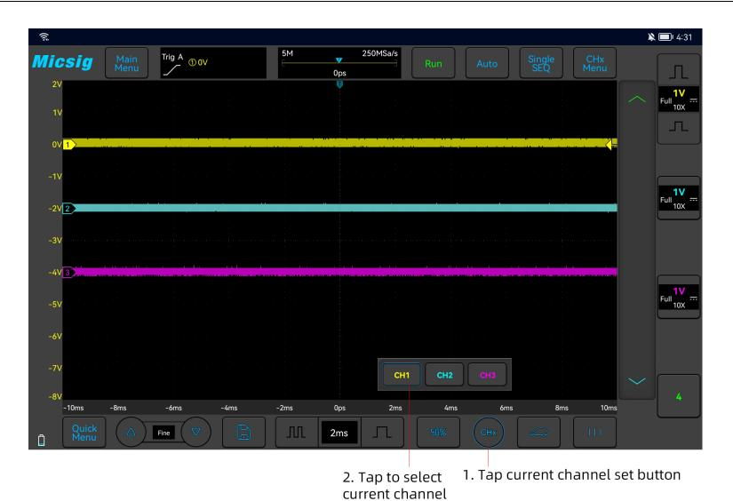
Figure 5-5 Using the Current Channel Selection Button
