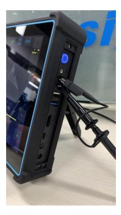
Figure 2-14 Probe Connection
