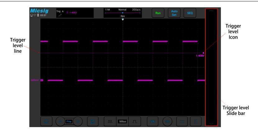
Figure 5-8 Trigger Level
