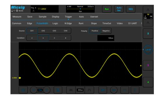
• Trigger condition and pulse width time: "greater than", the adjustment time is 180us.
