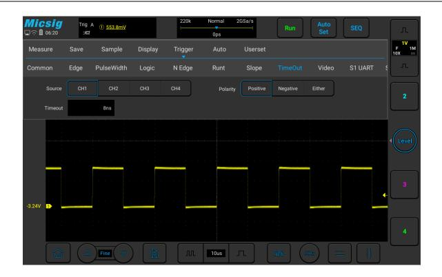
Figure 5-29 Time-out Trigger
