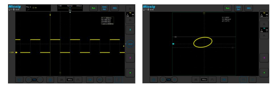
Figure 6-18 Cursor Measurement Pulse Width
