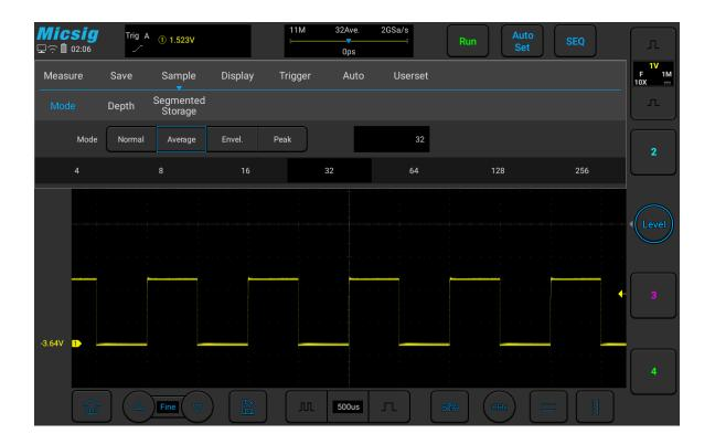
Figure 10-7 Waveform after choosing the average sampling mode, with average number 32
