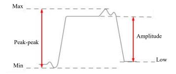
Figure 6-7 Voltage Measurement
