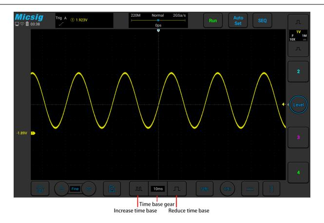
Figure 3-3 Adjust the Horizontal Time Base
