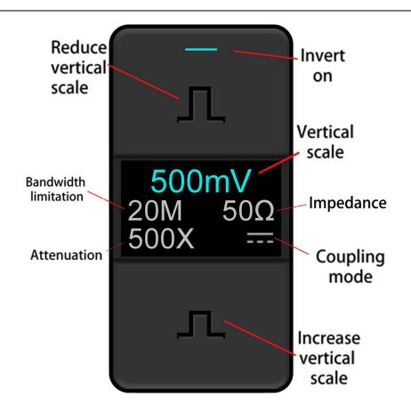
Figure 4-3 Channel Display Interface
