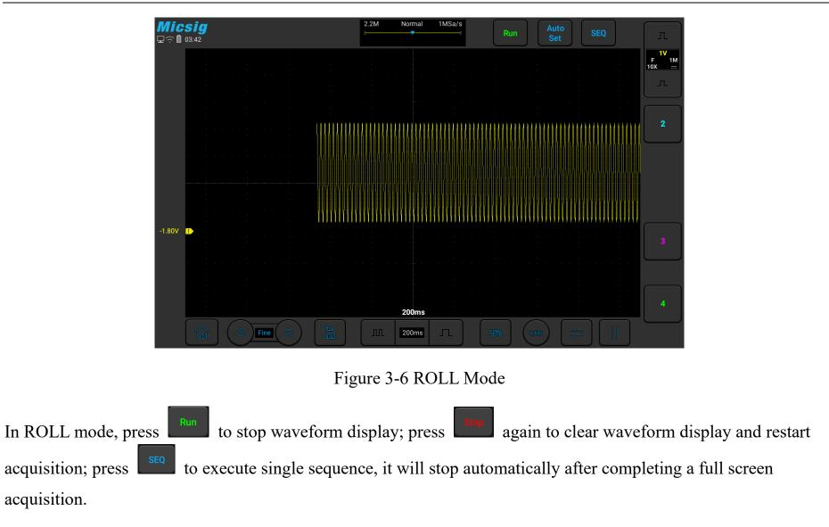
ROLL mode is generally used to observe waveforms with frequencies below 5 Hz.
