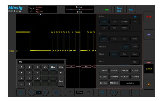
Figure 11-5 Baud Rate Default Setting
