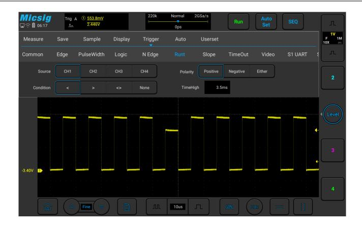
Figure 5-25 Runt Trigger Setting Menu
