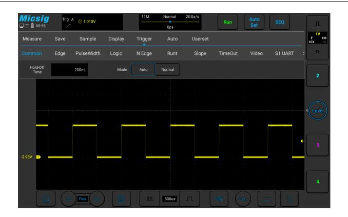
Figure 5-5 Oscilloscope Trigger Mode Setting
