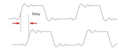
Figure 6-5 Delay Measurement Schematics
