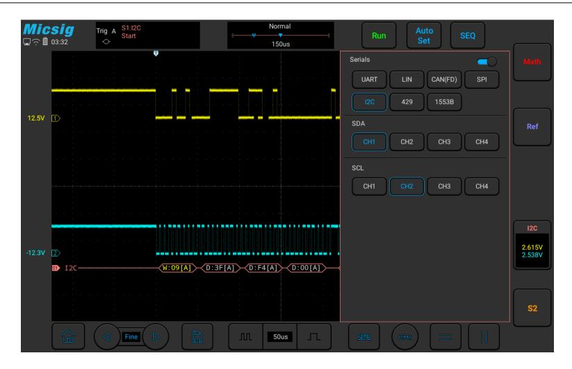
Figure 11-22 I2C Bus Configuration Menu
