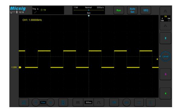
Figure 6-15 Frequency Meter Measurement
