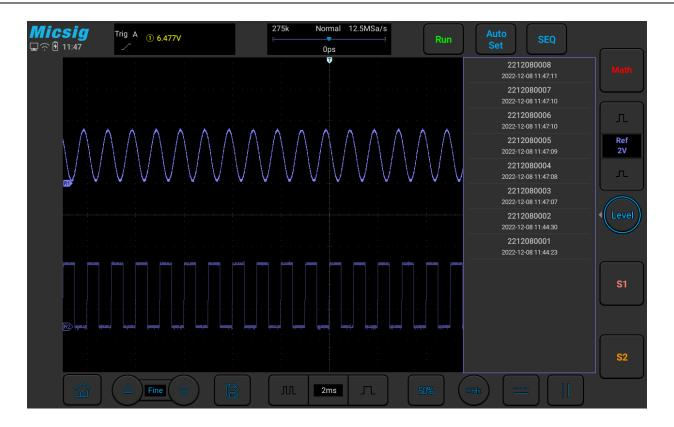
Figure 8-7 Restore Reference Waveform
