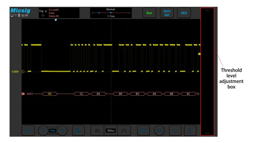
Figure 11-7 UART Decode Level Adjustment
