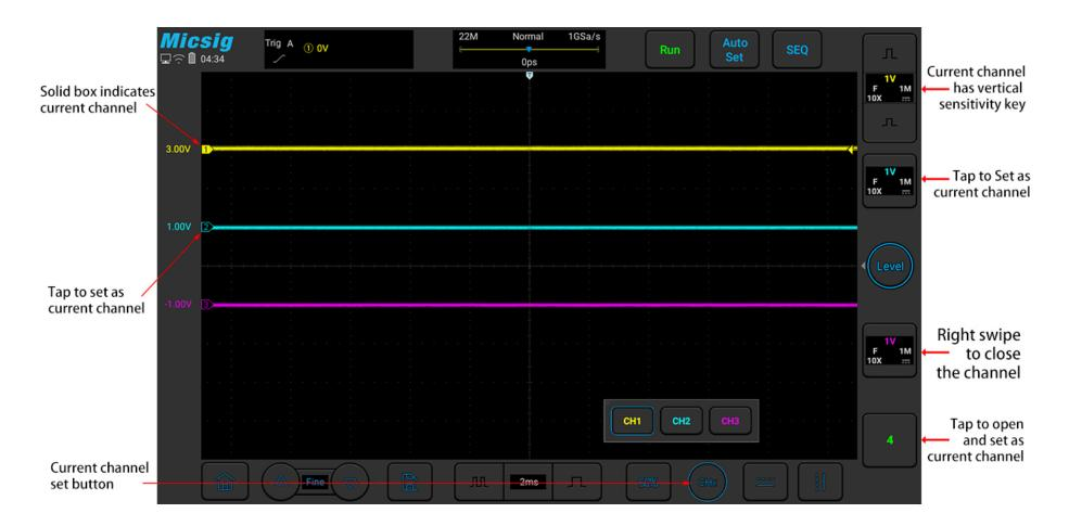
Figure 4-4 Channel Open, Close and Switching
