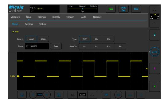
Figure 7-5 Save CH1 Reference Waveform Interface
