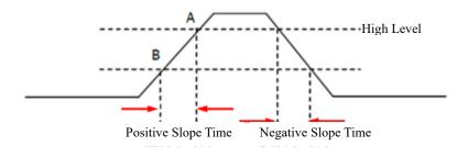
Figure 5-26 Positive/Negative Slope Time
