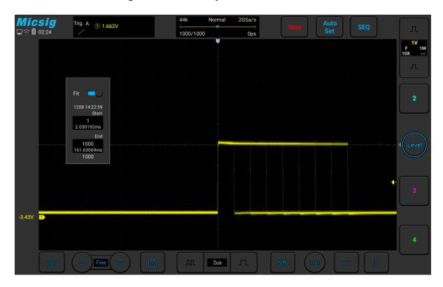
Figure 10-13 Segmented storage fitting view
