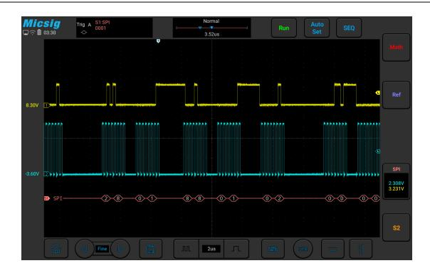
Figure 11-20 SPI Graphic Interface
