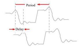
Figure 6-6 Phase Measurement Schematics
