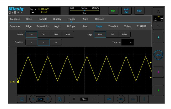
Figure 5-27 Slope Trigger Setting Menu
