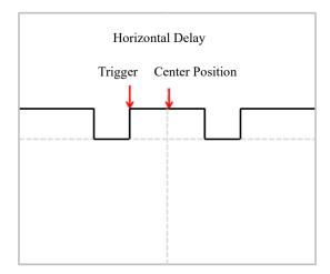
Figure 5-7 Horizontal Delay
