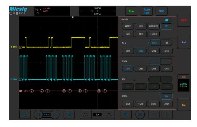
Figure 11-18 SPI Bus Configuration Menu
