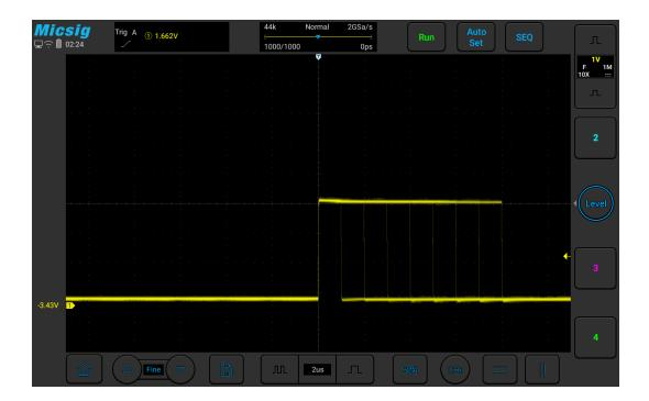
Figure 10-11 Segmented memory waveform acquisition
