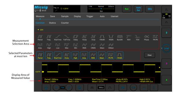
Figure 6-1 Automatic Measurement Menu
