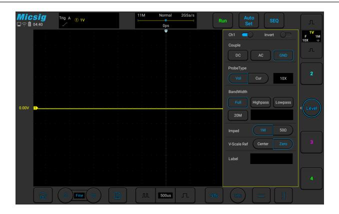
Figure 4-9 GND Coupling
