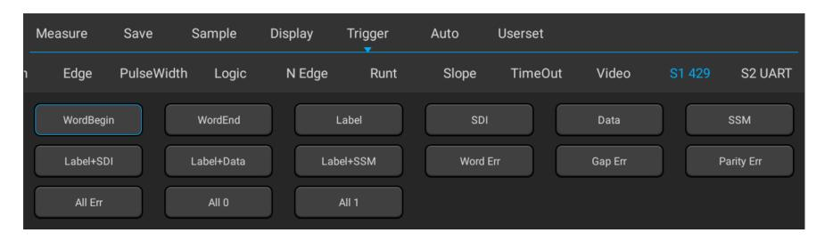
Figure 11-27 ARINC429 Trigger Mode Configuration Menu
