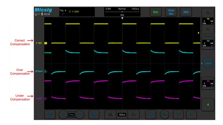
Figure 2-15 Probe Compensation
