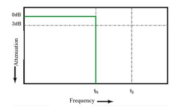
Figure 10-2 Theoretical Brick-Wall Frequency Response
