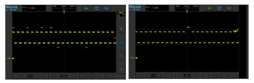
Figure 5-3 Abnormal Signal in Periodic Signals
