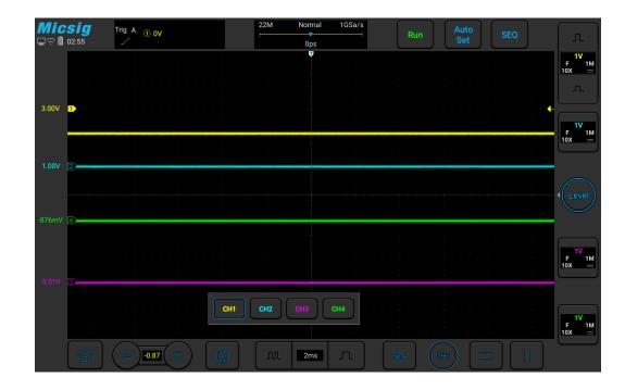
Figure 2-13 Manual zero calibration
