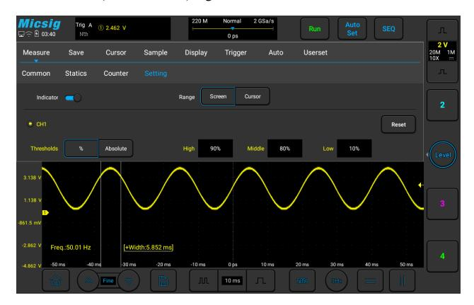
Figure 6-13 Set Middle Thresholds as 80%
