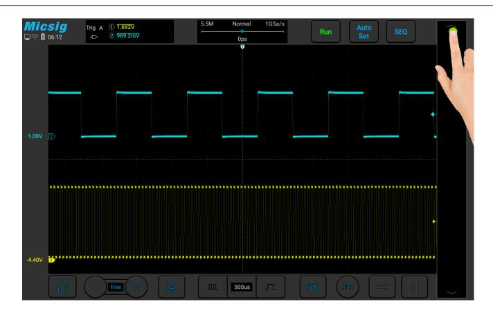
Figure 5-22 Trigger Level Adjustment
