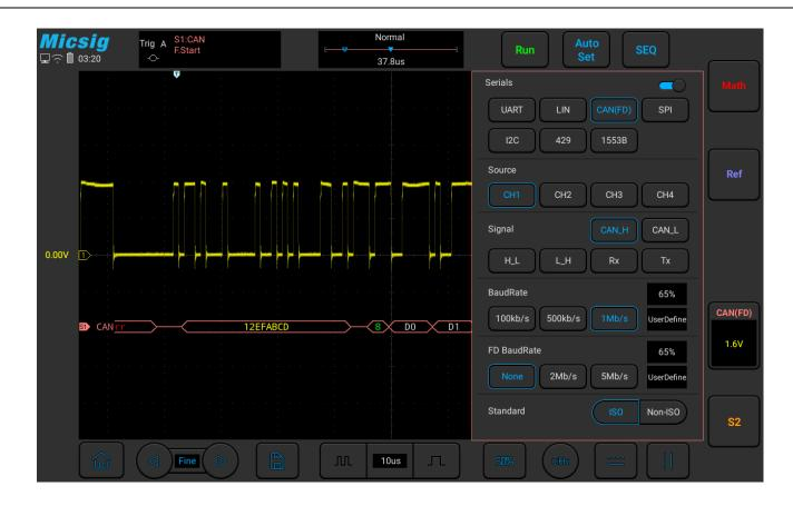
Figure 11-14 CAN(FD) Bus Configuration Menu
