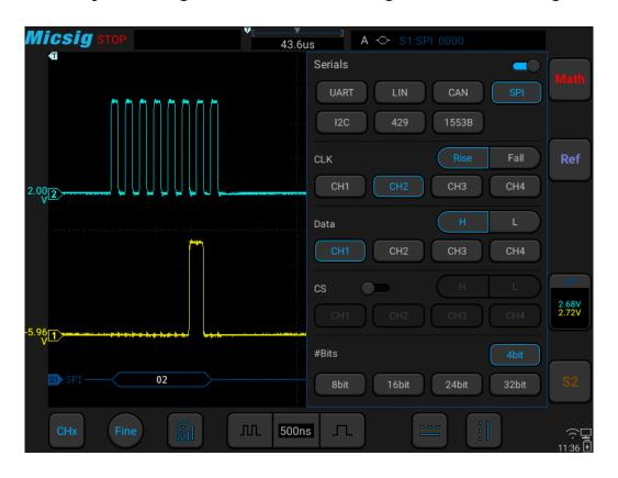
Figure 12-18 SPI Bus Configuration Menu
