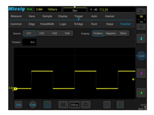
Figure 6-29 Time-out Trigger
