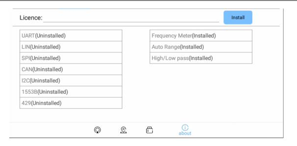
Figure 15-2 Decode Functions Not Installed
