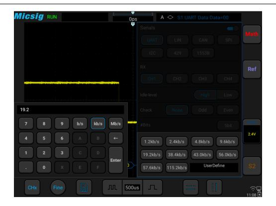
Figure 12-5 Baud Rate Default Setting
