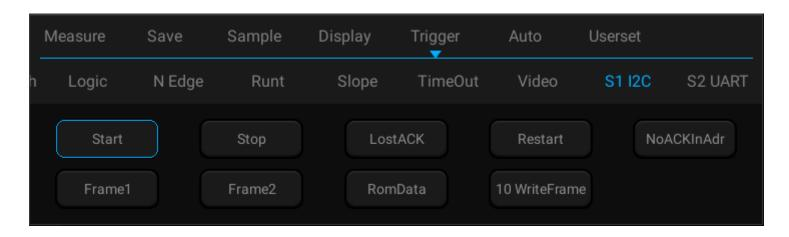
Figure 12-23 I2C Trigger Mode Configuration Menu
