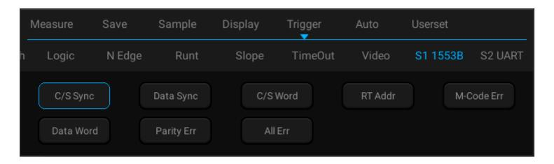
Figure 12-31 1553B Trigger Mode Configuration Menu
