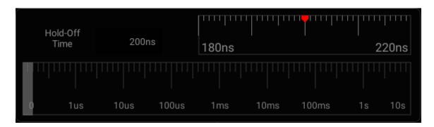
Figure 6-11 Trigger Hold-Off Time Set Interface
