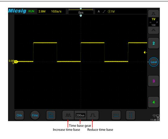
Figure 4-3 Adjust the Horizontal Time Base
