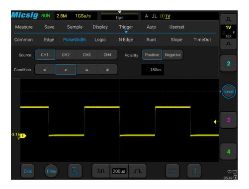
Figure 6-14 Pulse Width Trigger Setting Menu
