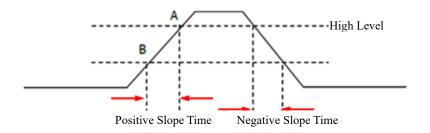
Figure 6-26 Positive/Negative Slope Time
