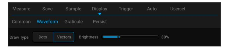
Figure 10-2 Waveform Display Menu
