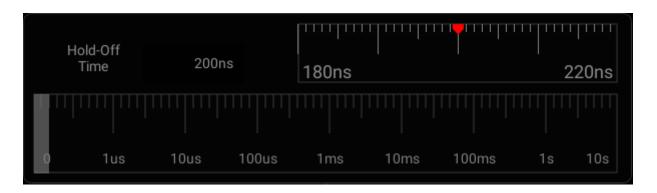
Figure 3-2 Trigger hold-off time
