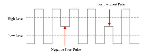
Figure 6-24 Runt Trigger
