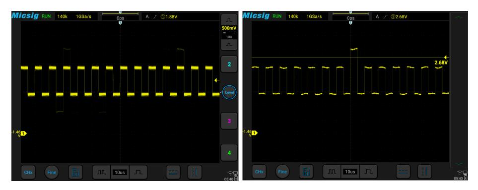
Figure 6-3 Abnormal Signal in Periodic Signals
