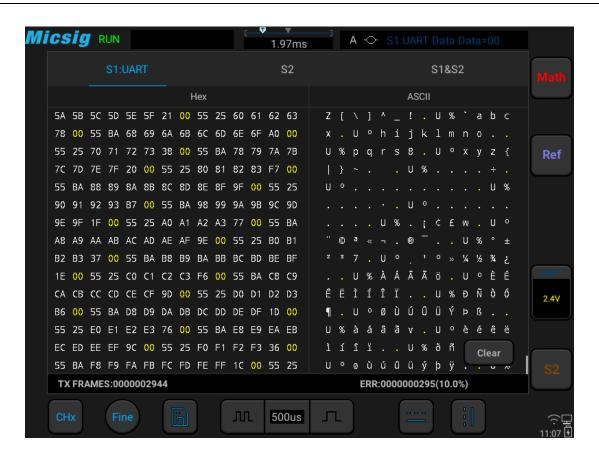
Figure 12-2 Bus Decode Text Mode
