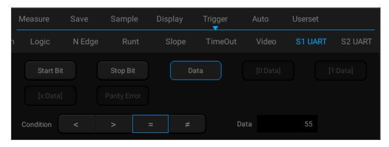
Figure 12-6 Trigger Setting Menu
