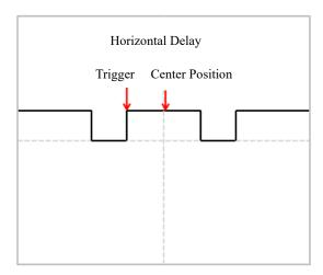
Figure 6-7 Horizontal Delay
