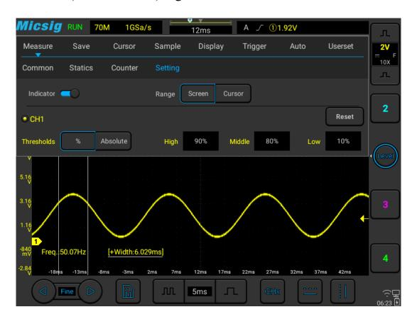
Figure 7-13 Set Middle Thresholds as 80%
