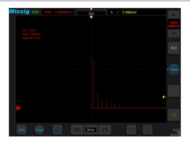
Figure 9-4 Spectrum Amplitude as V-Hz
