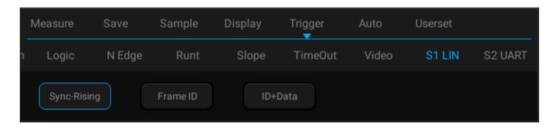
Figure 12-11 LIN Trigger Mode Configuration Menu
