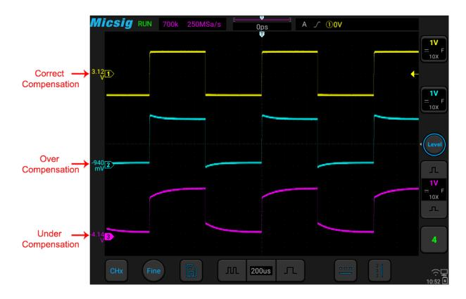
Figure 2-14 Probe Compensation
