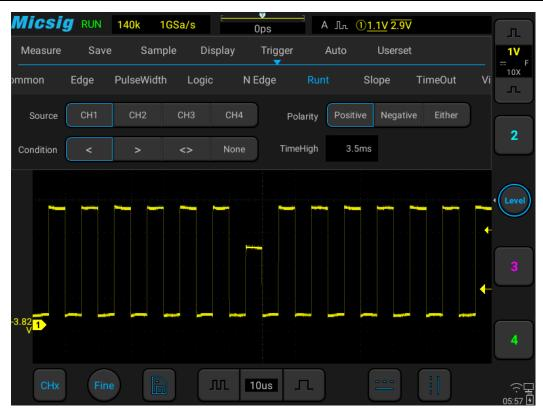
Figure 6-25 Runt Trigger Setting Menu
