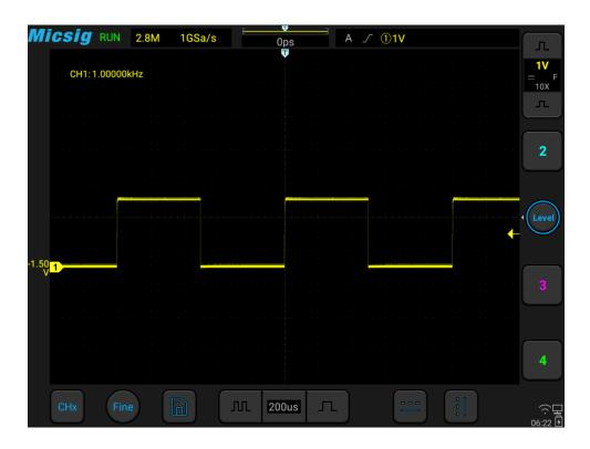
Figure 7-15 Frequency Meter Measurement
