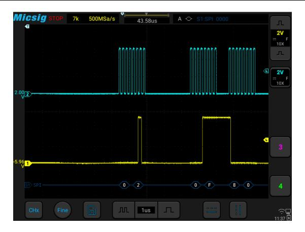
Figure 12-20 SPI Graphic Interface
