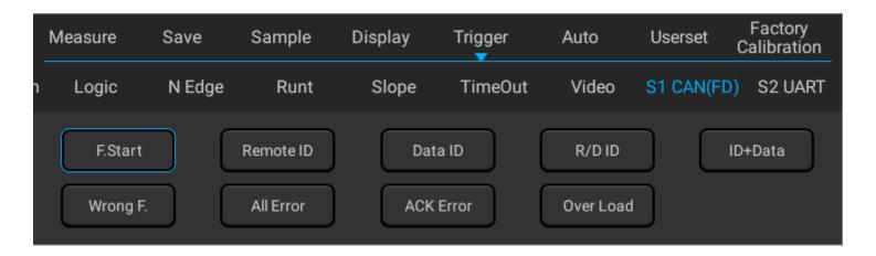
Figure 12-15 CAN Trigger Mode Configuration Menu
