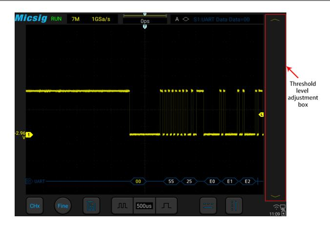
Figure 12-7 UART Decode Level Adjustment
