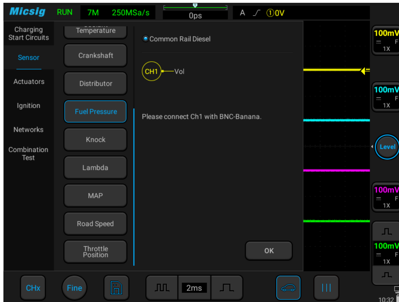
Figure 3-18 Fuel Pressure Sensor Test
