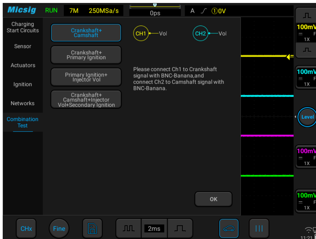
Figure 3-50 Crankshaft + Camshaft Combination Test
