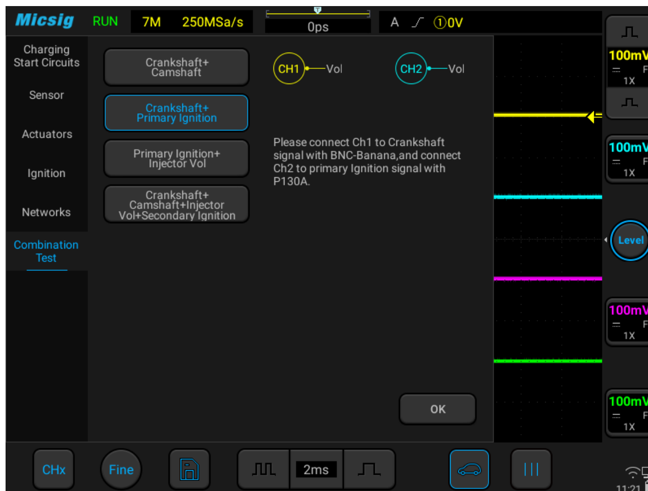
Figure 3-51 Crankshaft + Primary ignition test
