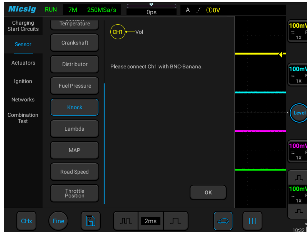
Figure 3-19 Knock Sensor test
