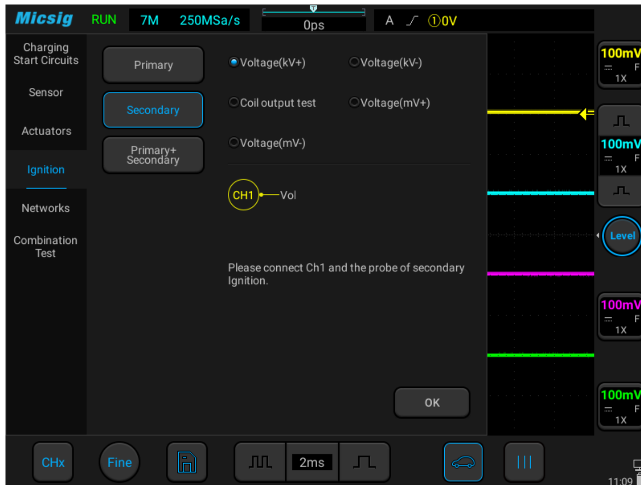
Figure 3-42 Secondary ignition test
