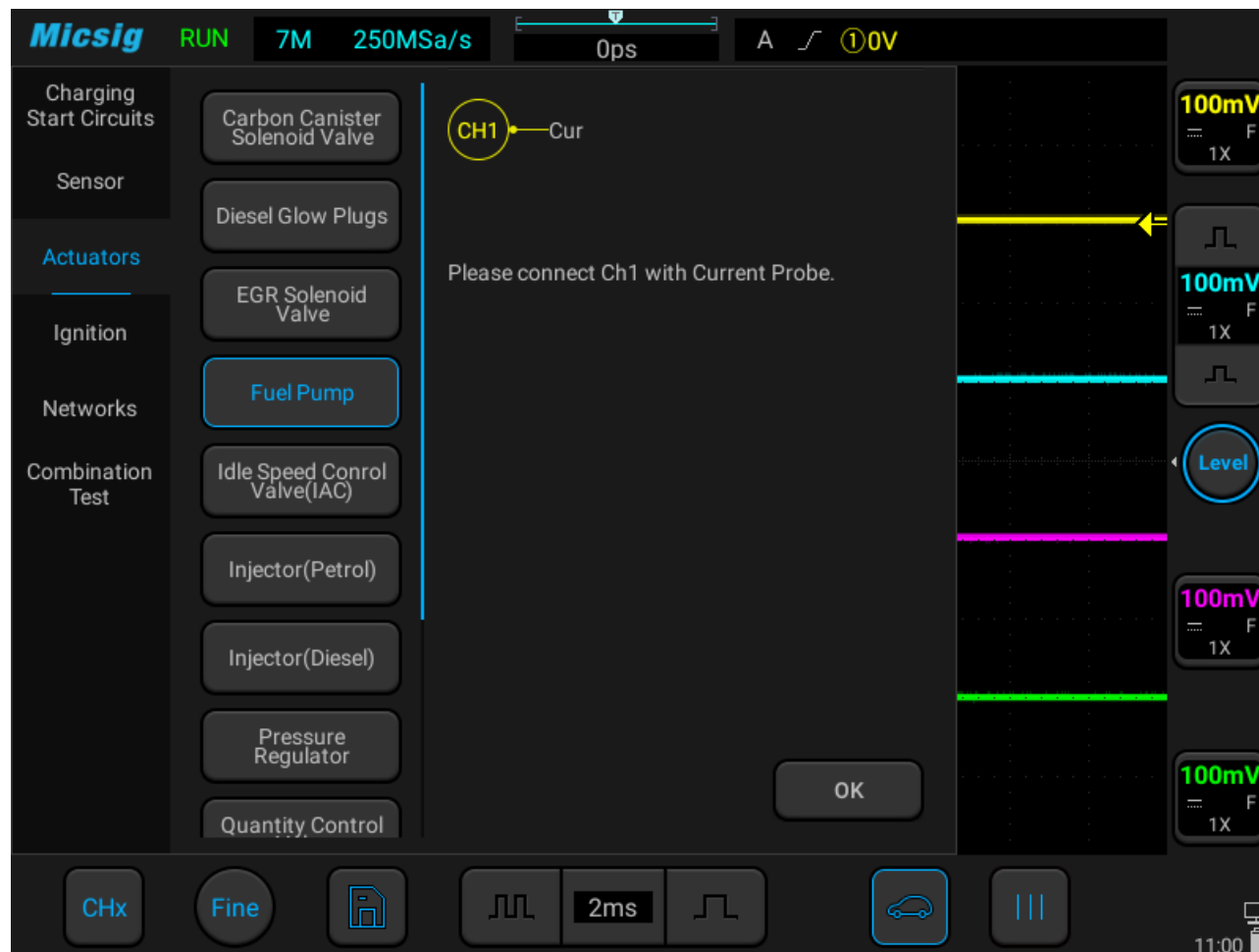
Figure 3-30 Electronic fuel pump test
