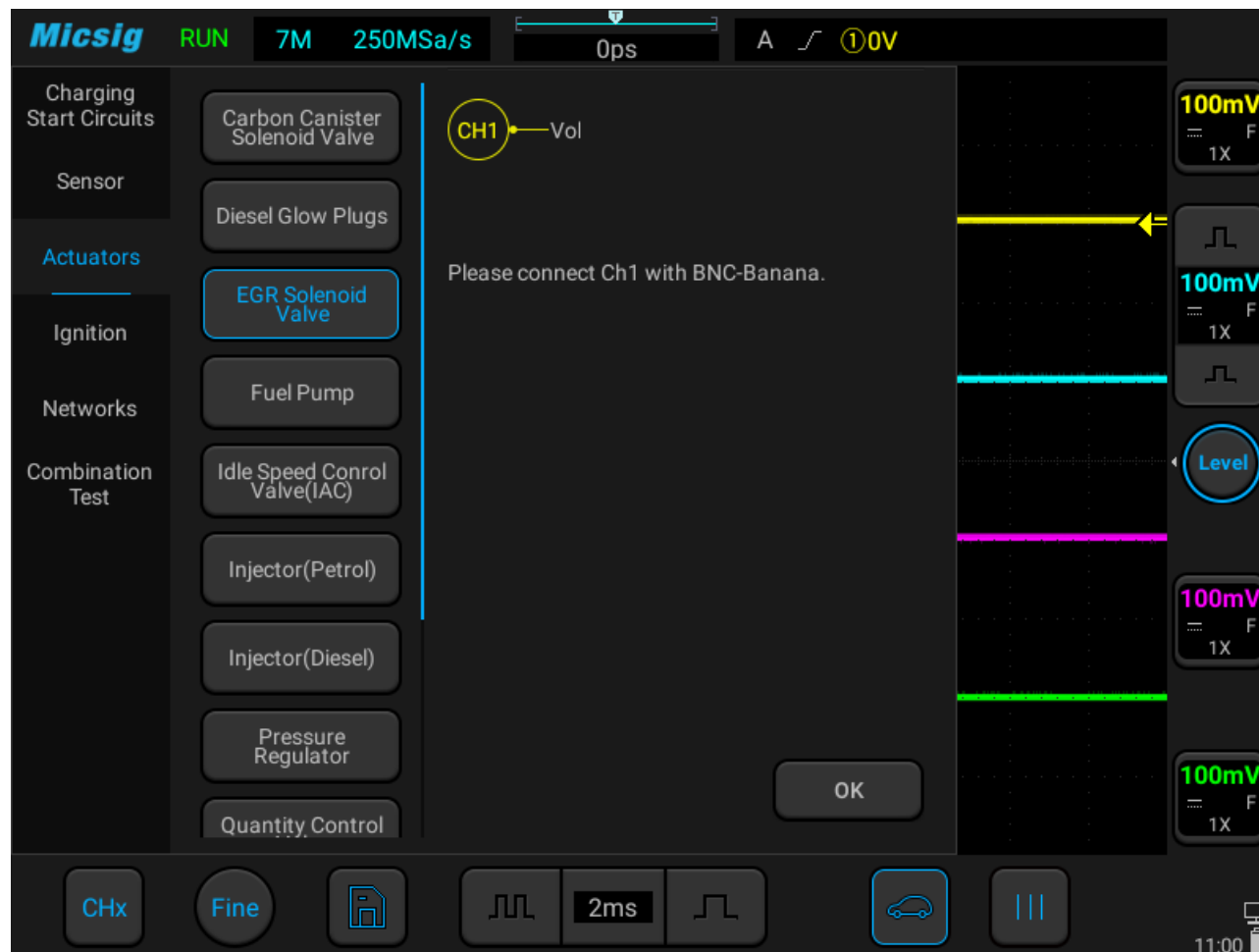
Figure 3-29 EGR solenoid valve test
