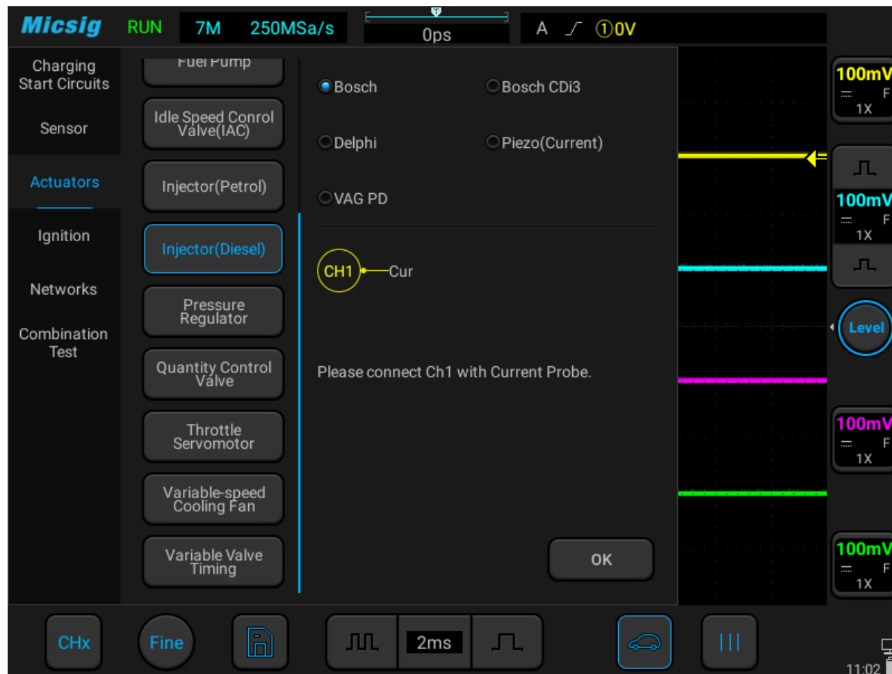
Figure 3-33 injector (diesel engine) test
