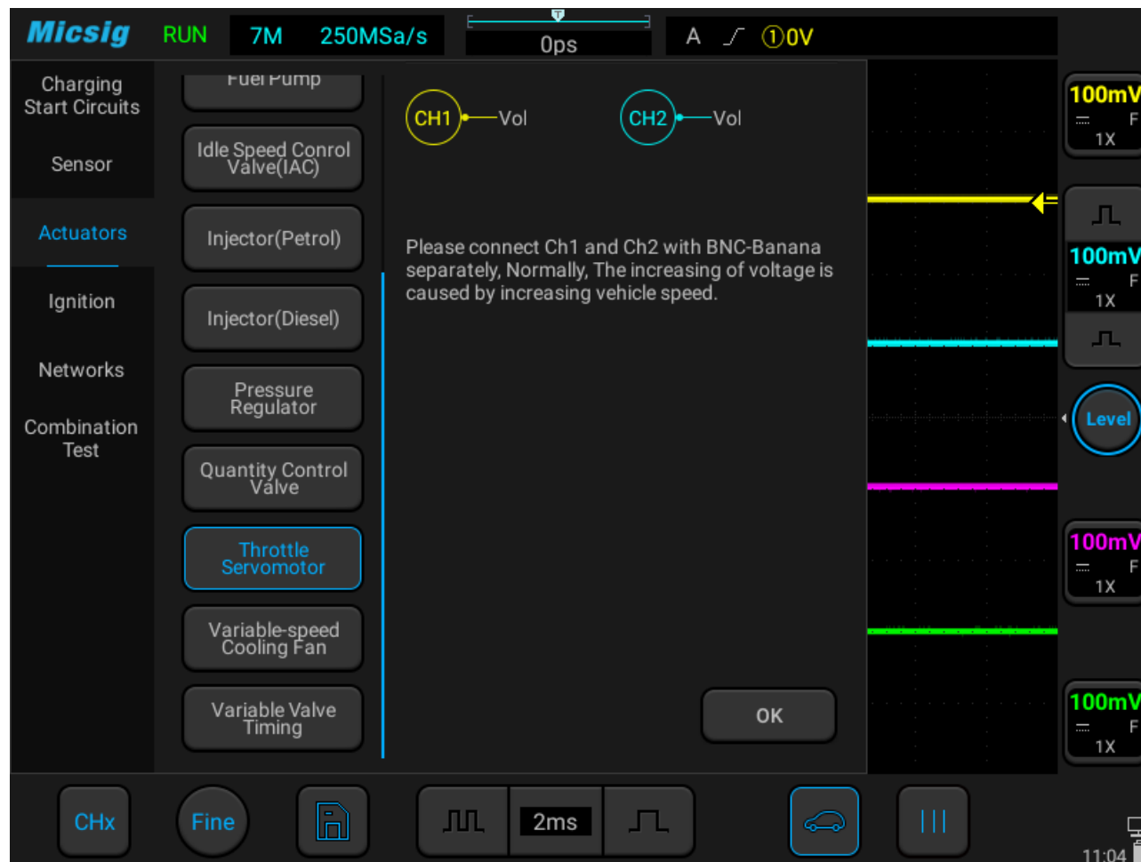
Figure 3-36 Throttle servo motor test
