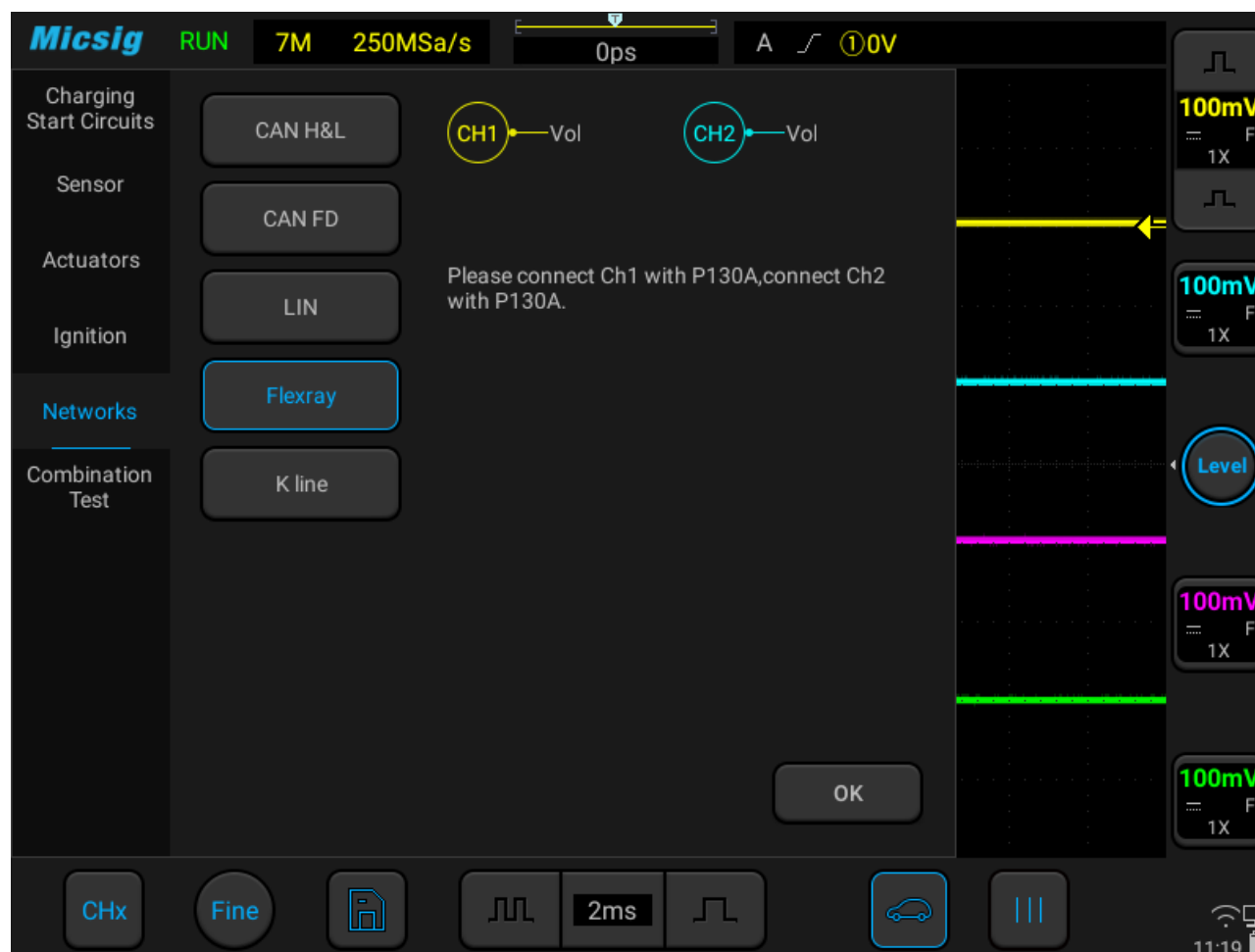
Figure 3-48: FlexRay bus test
