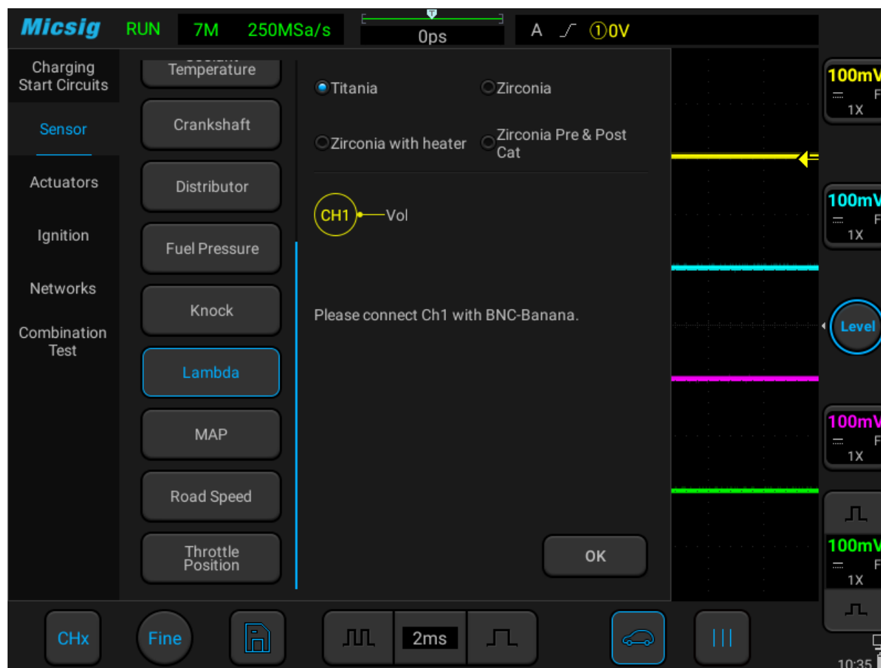
Figure 3-20 Lambda (oxygen sensor) test
