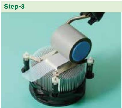
Roll twice on the film to attach to heat sink
