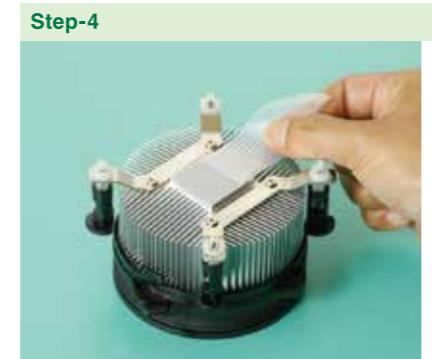
Peel off instantly the PET film to horizontal direction
