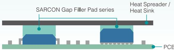
In areas where space between surface is uneven or varies and where surface textures are a concern regarding efficient thermal transfer, the supple consistency of Gap Filler Pad is excellent for filling air gaps and uneven surfaces.
