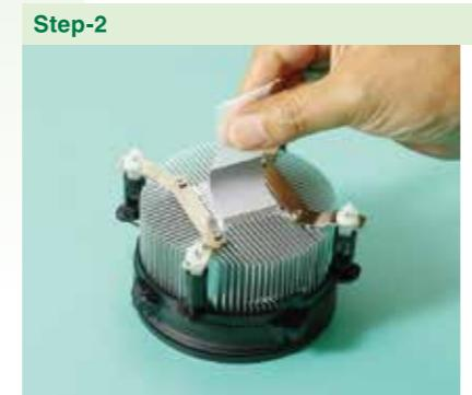
Apply onto Heat Sink
