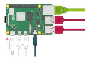
You should see a red LED light up on the Raspberry Pi, which indicates that Raspberry Pi is connected to power. As it starts up (this is also called booting), you will see raspberries appear in the top left-hand corner of your screen.
