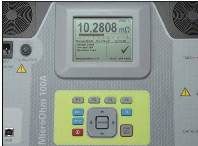
Figure 4.1: Display and keyboard layout
