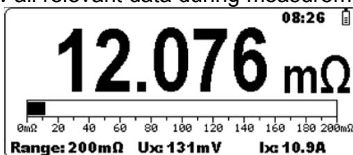
Figure 4.7: Measurement window
