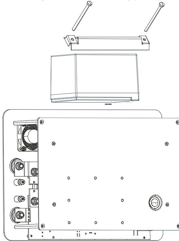
5. Replace battery (use Panasonic LC-CA1212P1 or similar) and reassemble the instrument.
