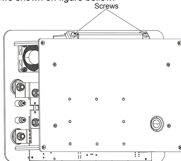
4. Remove screws, battery holder and carefully pull out battery.
