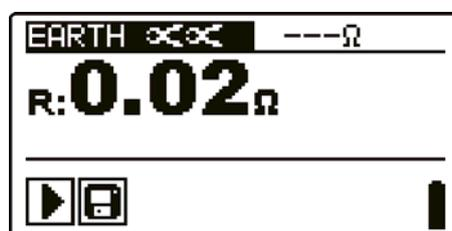
Figure 5.8: Example of contactless earthing resistance measurement result
