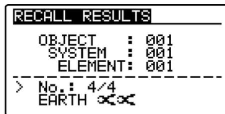
Figure 6.4: Recall menu - measurements field selected
