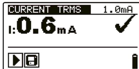
Figure 5.13: Example of clamp current measurement result
