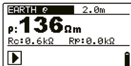
Figure 5.10: Example of specific earth resistance measurement result
