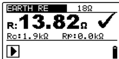
Figure 5.4: Example of earth resistance measurement result
