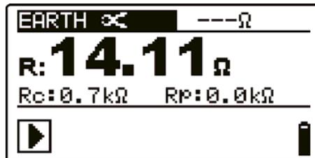
Figure 5.6: Example of selective earth resistance measurement results
