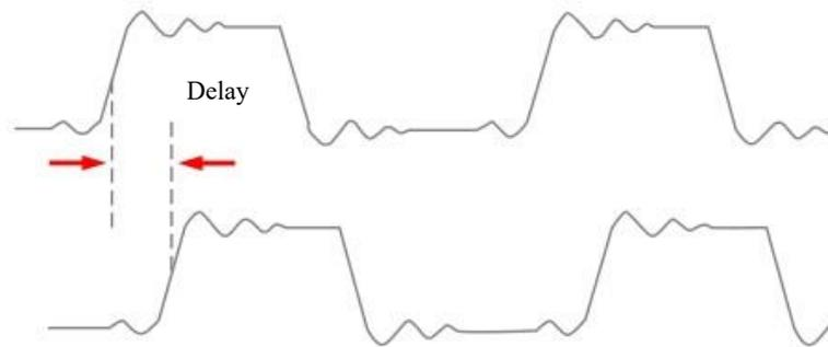
Figure 7-5 Delay Measurement Schematics
