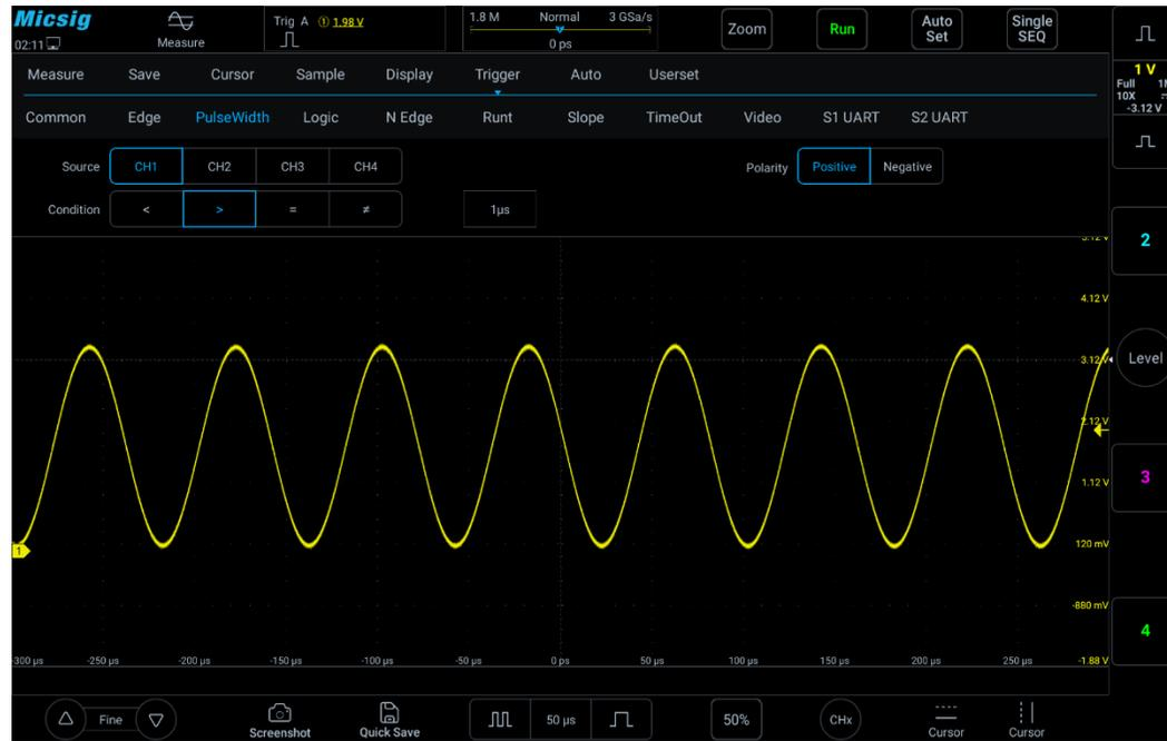
Figure 6-14 Pulse Width Trigger Setting Menu
