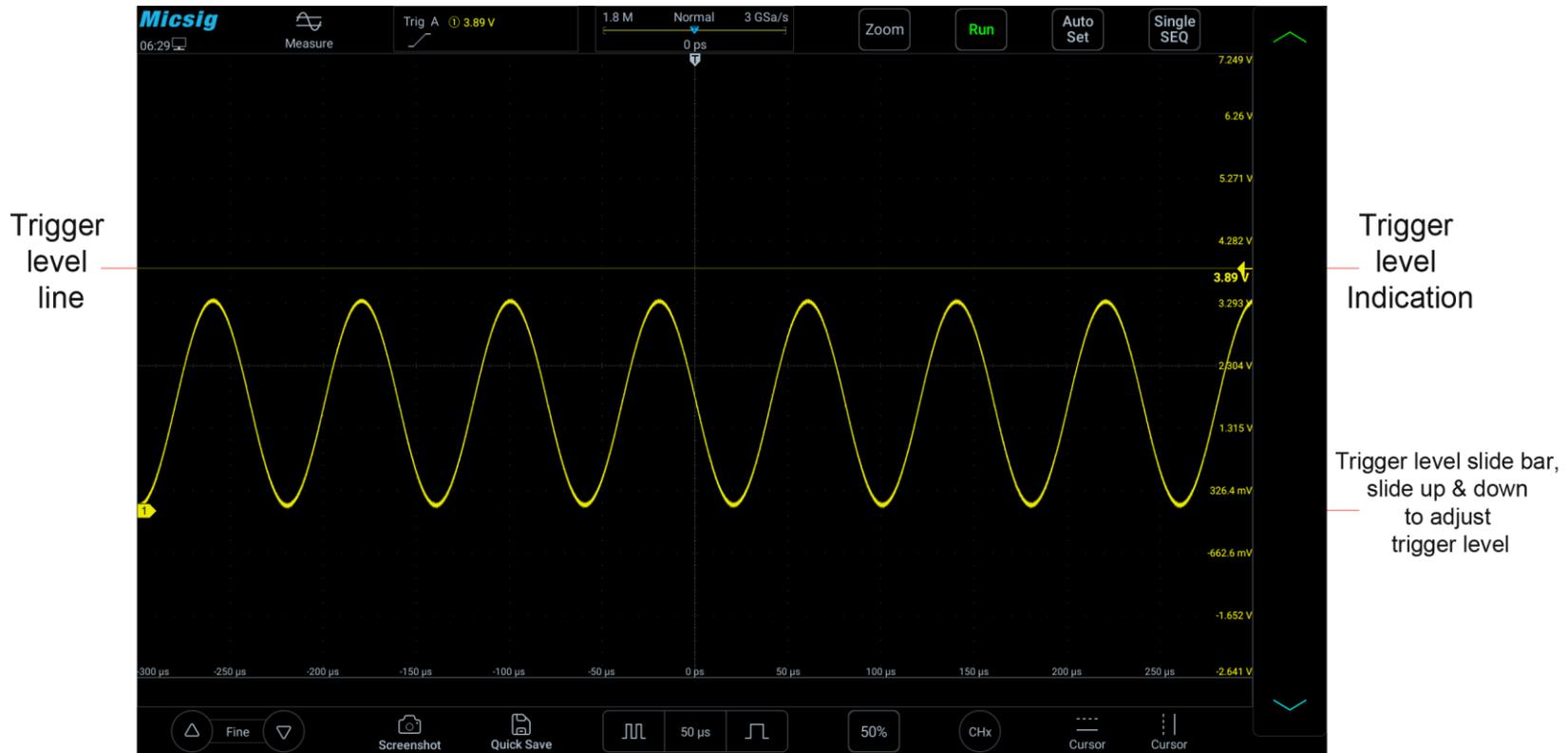
Figure 6-8 Trigger Level
