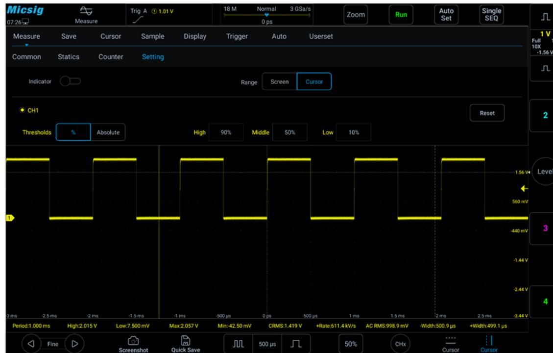
Figure 7-9 Automatic measurement range selection as cursor
