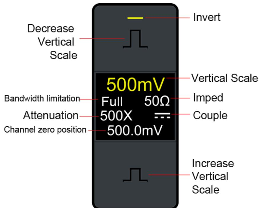
Figure 5-3 Channel Display Interface
