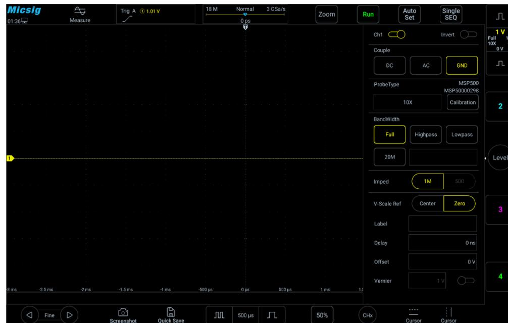
Figure 5-9 GND Coupling
