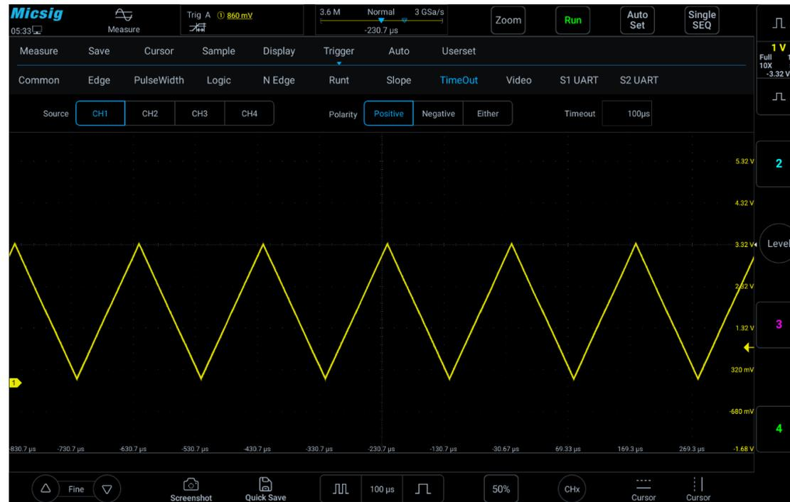
Figure 6-29 Time-out Trigger
