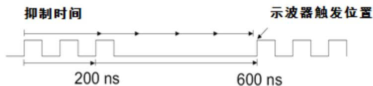
Figure 6-10 Trigger Hold-Off Time
