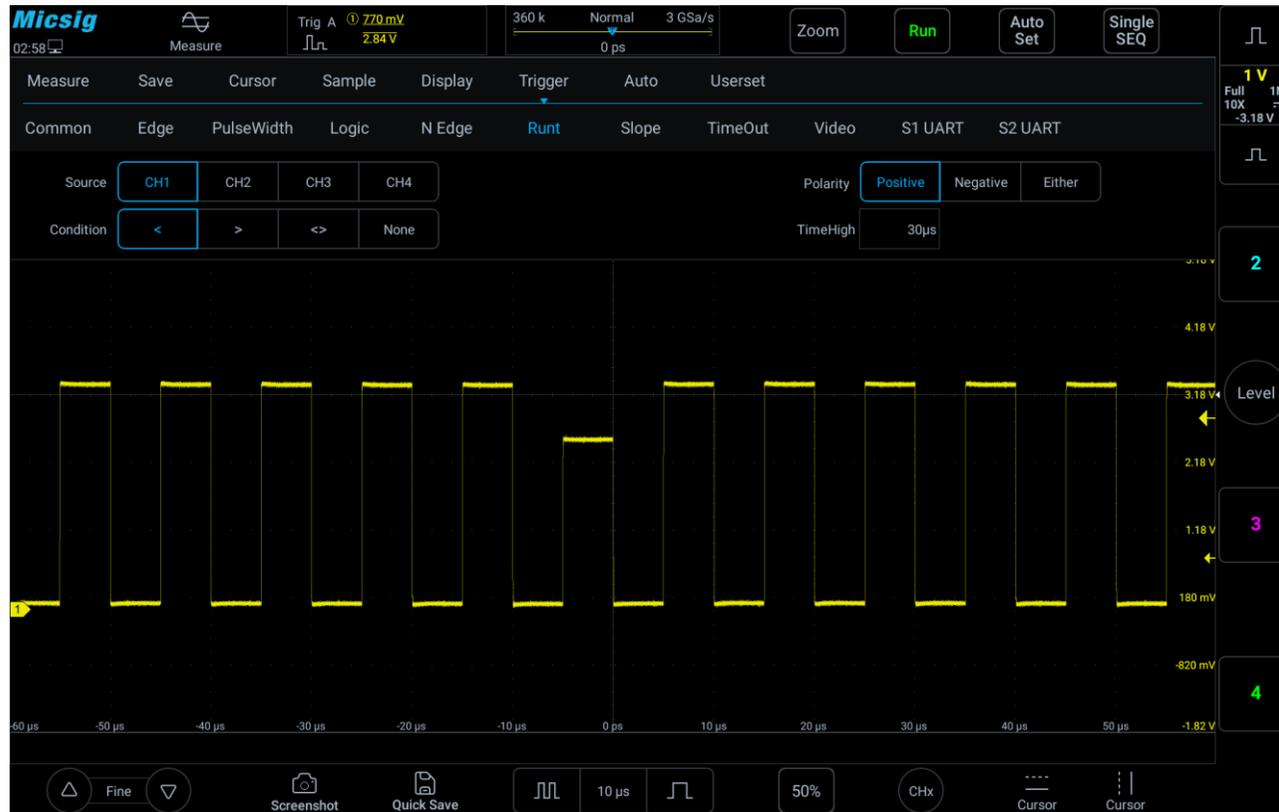
Figure 6-25 Runt Trigger Setting Menu
