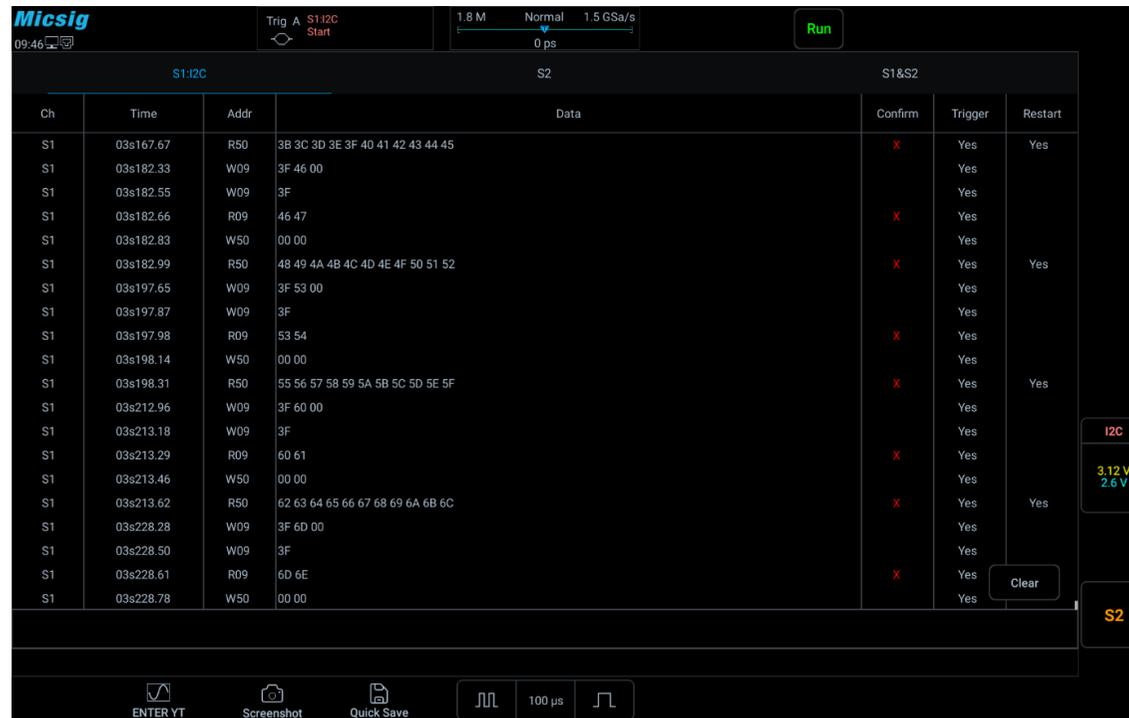
Figure 12-25 I<sup>2</sup>C Text Interface
