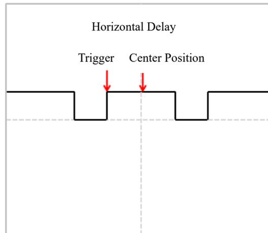
Figure 6-7 Horizontal Delay
