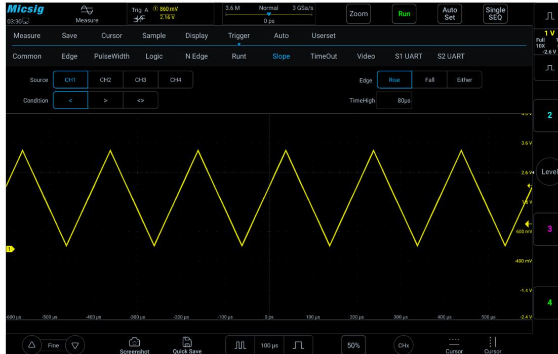
Figure 6-27 Slope Trigger Setting Menu
