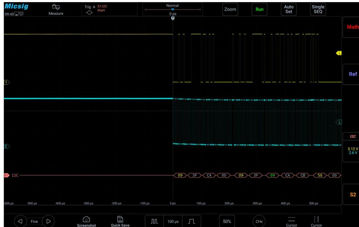
Figure 12-24 I<sup>2</sup>C Graphic Interface
