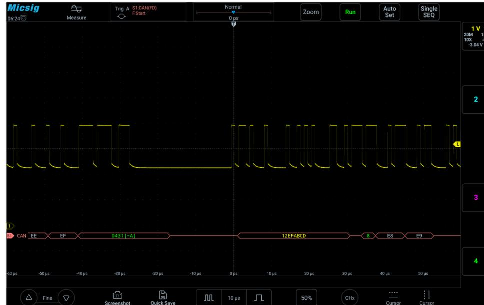
Figure 12-16 CAN bus decode interface
