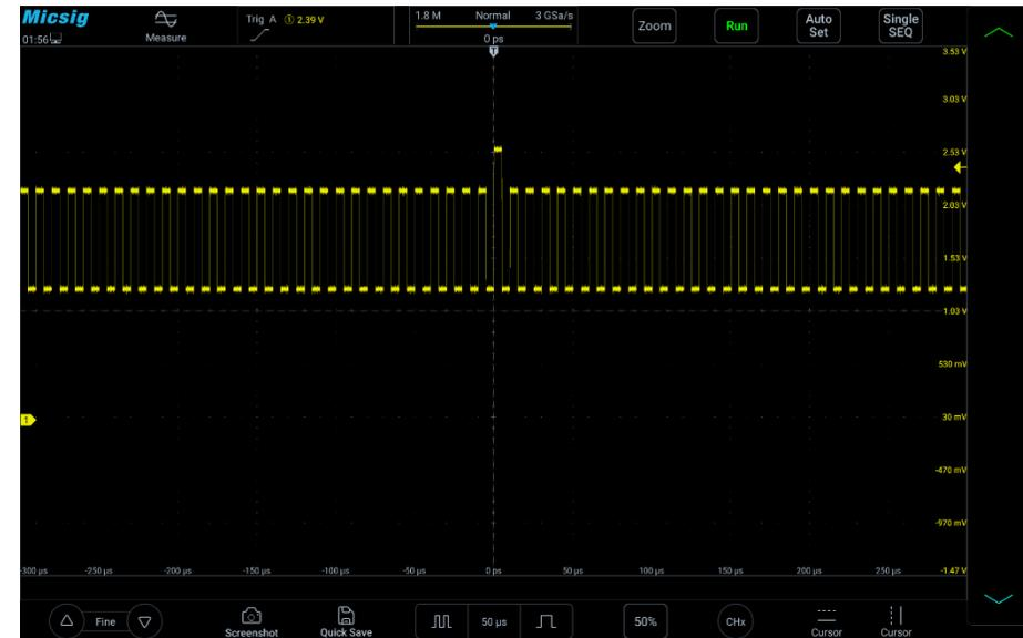
Figure 6-4 Abnormal Signal Captured by Setting Trigger Level
