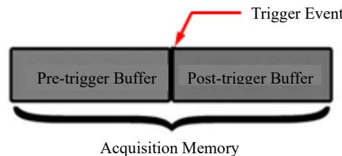
Figure 6-6 Conceptual Demonstration of Acquisition Memory
