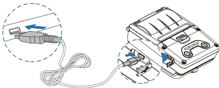
Connect the USB cable to the PC to charge the printer.
