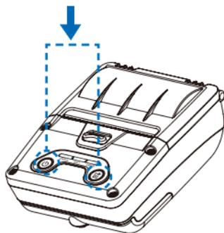
While you are holding the FEED button, press the power button.
