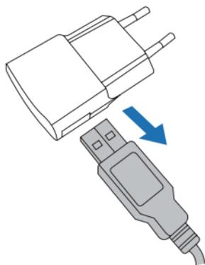
Disconnect the USB cable from the power cord adapter.
