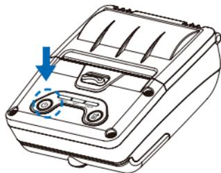
Turn off the power by pressing the power button for approximately 3 seconds.
