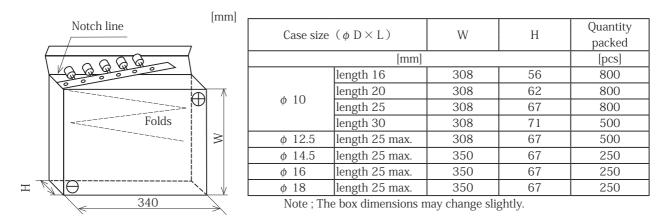
% For  $\phi$  10 and  $\phi$  12.5 with P=15, the capacitors located on folds shall be removed. (The polarity orientation does not apply to non-polarized capacitors.)
