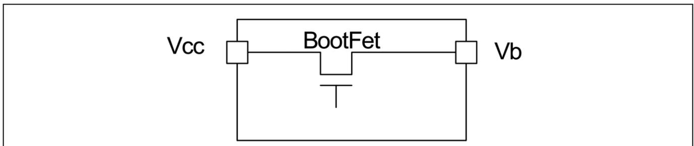
Figure 22 Simplified BootFET internal connection
