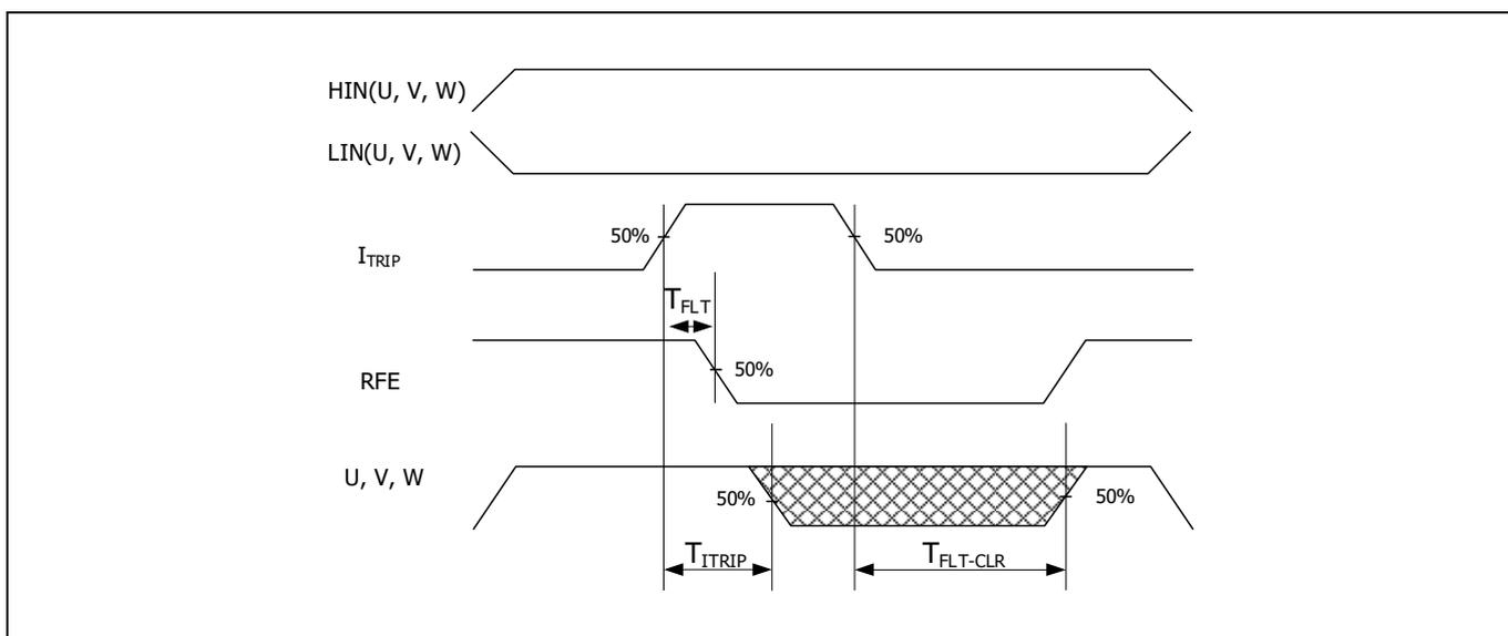
**Figure 9** Timing chart for the overcurrent protection function
