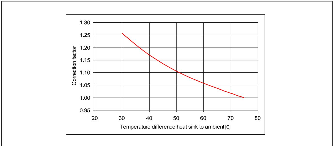
Figure 31 Correction factors for temperature
