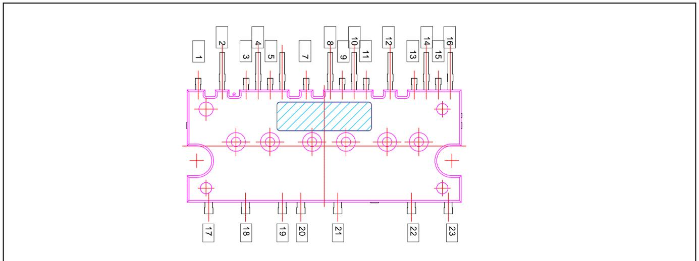
Figure 4 Module pinout
