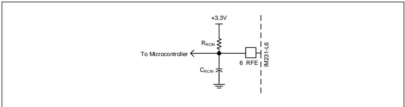
**Figure 11** Typical PCB circuit connected to the RFE pin
