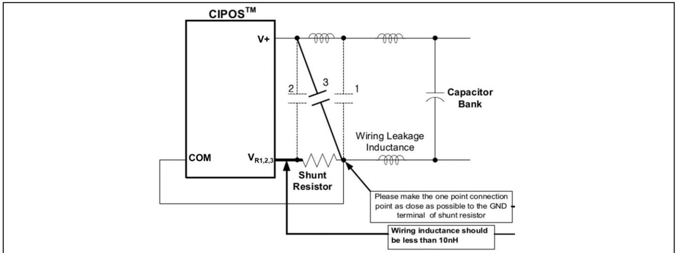
**Figure 20** Proper snubber capacitor use
