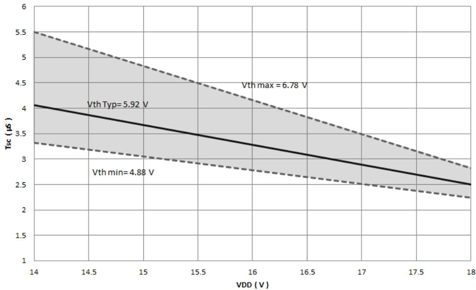
Figure 10 IM231-x6 t<sub>SC</sub> vs V<sub>DD</sub> with V<sub>DC</sub> = 400 V and T<sub>J</sub> = 150°C
