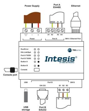
Power Supply Must use NEC Class 2 or Limited Power Source (LPS) and SELV rated power supply.
