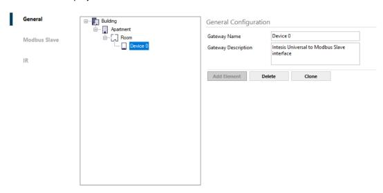
To modify the name of an element of the tree, click on it and edit it on the right side\*. It is also possible to add a description of a gateway for the integrator reference.
