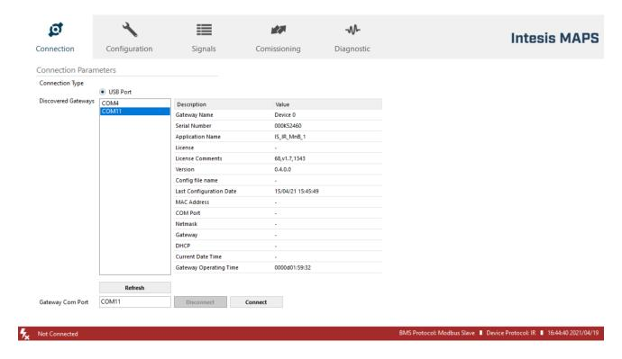
Connect to the device using Connect button. Once the software is connected to the interface, the lower bar will indicate is as shown in the image, and the product LED will turn into intense steady orange:
