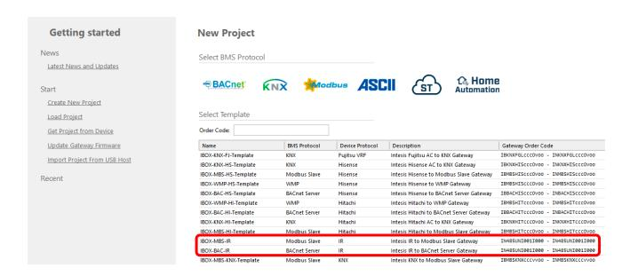
Remember that the product doesn't communicate in both protocols at the same time (BACnet/Modbus) and is not intended for a quick change of the communication protocol. However, is possible to change between BACnet and Modbus protocols by downloading a configuration done in a different template.
