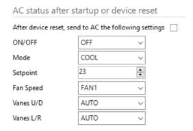
After device reset, send to AC the following settings (active/not active): by activating this function, the interface will send the following AC status to the AC unit in case the device booted for any reason.
