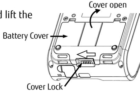
2. Set the battery and slide to battery terminal side for battery locking.
