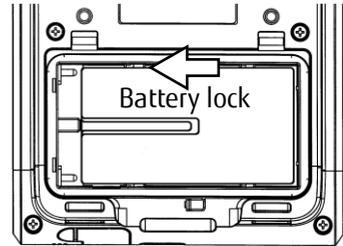
3. Please hook battery cover on the battery insertion area and push the battery cover to close.
