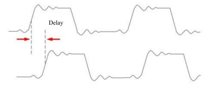
Figure 6-5 Delay Measurement Schematics
