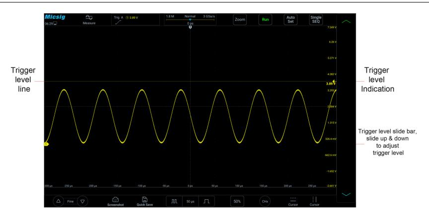
Figure 5-8 Trigger Level
