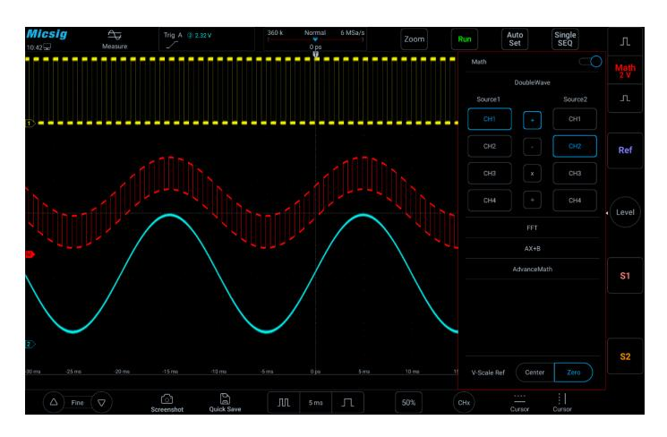
Figure 8-1 MATH Channel Waveform
