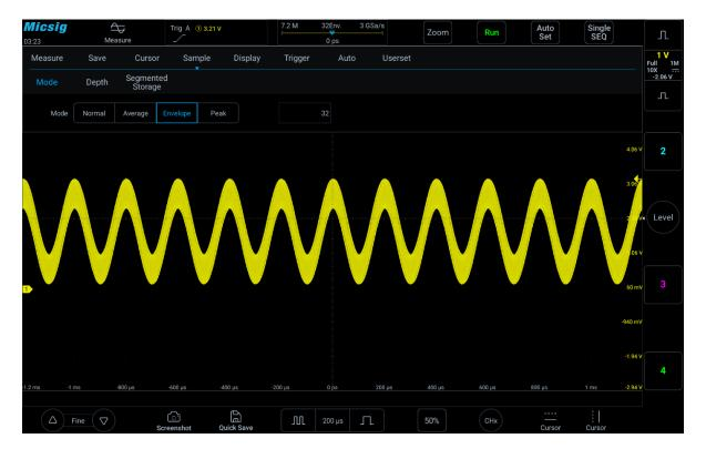
Figure 10-8 Signal in Envelope Sampling Mode (32)
