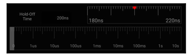
Figure 5-11 Trigger Hold-Off Time Set Interface
