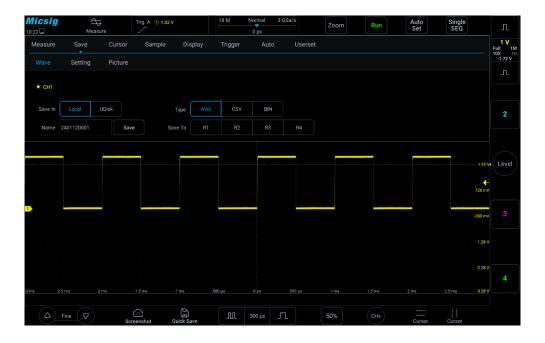
Figure 7-5 Save CH1 Reference Waveform Interface
