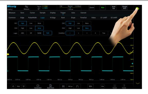
Figure 5-22 Trigger Level Adjustment
