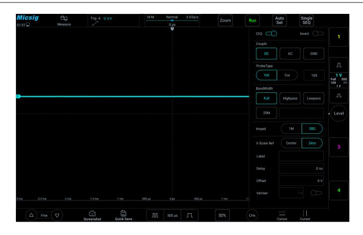
Figure 4-17 Channel input impedance
