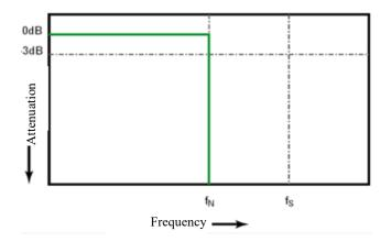
Figure 10-2 Theoretical Brick-Wall Frequency Response
