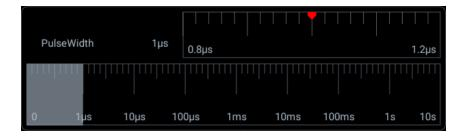
Figure 5-20 Pulse Width Time Adjustment Interface
