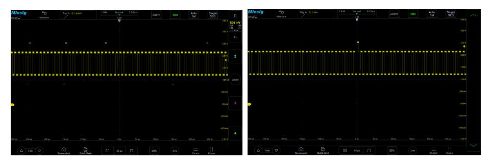
Figure 5-3 Abnormal Signal in Periodic Signals
