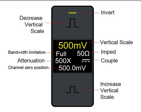
Figure 4-3 Channel Display Interface
