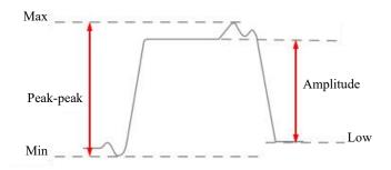
Figure 6-7 Voltage Measurement
