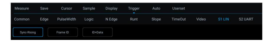
Figure 11-11 LIN Trigger Mode Configuration Menu
