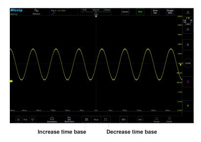
Figure 3-2 Adjust the Horizontal Time Base
