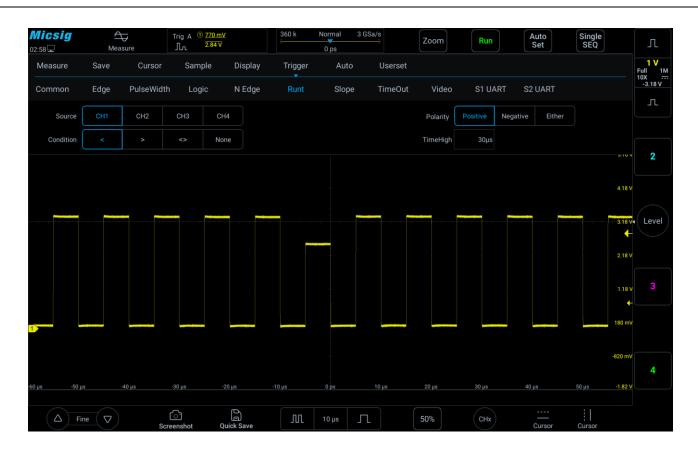
Figure 5-25 Runt Trigger Setting Menu
