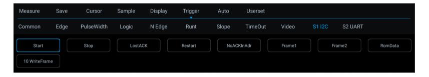
Figure 11-23 I<sup>2</sup>C Trigger Mode Configuration Menu
