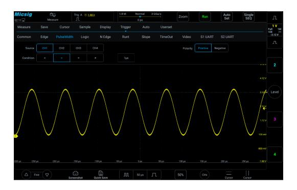
Figure 5-14 Pulse Width Trigger Setting Menu
