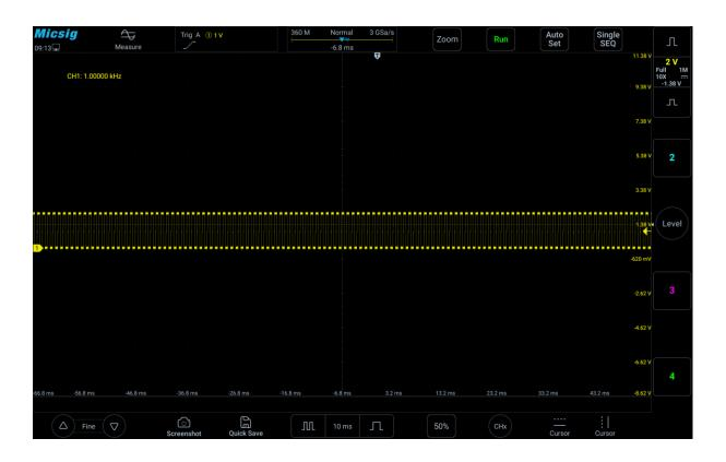
Figure 6-15 Frequency Meter Measurement
