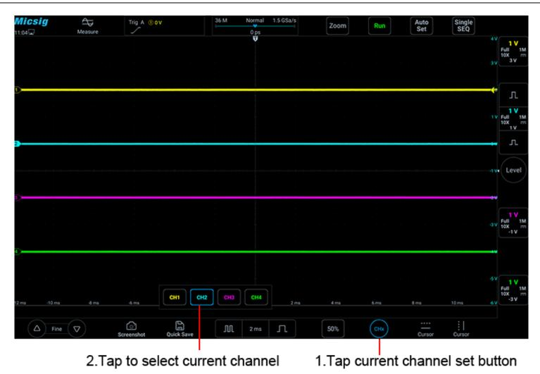
Figure 4-5 Using the Current Channel Selection Button
