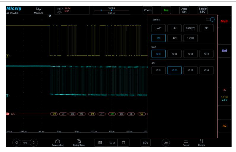
Figure 11-22 I<sup>2</sup>C Bus Configuration Menu
