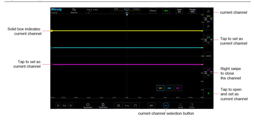
Figure 4-4 Channel Open, Close and Switching
