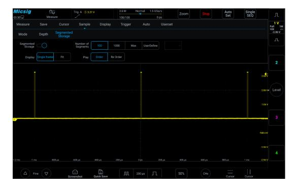
Figure 10-11 Segmented storage waveform acquisition
