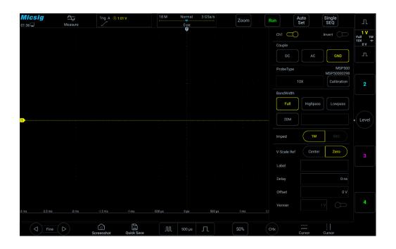
Figure 4-9 GND Coupling
