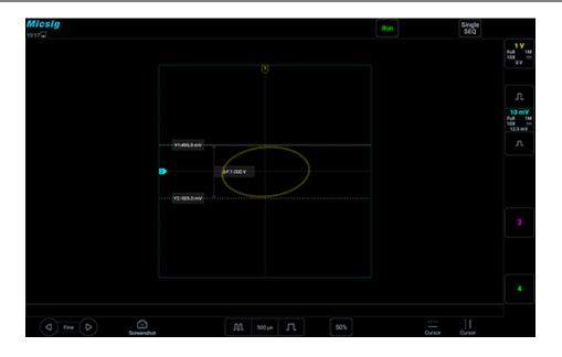
Figure 3-9 Phase Difference Measurement and Using the Cursor
