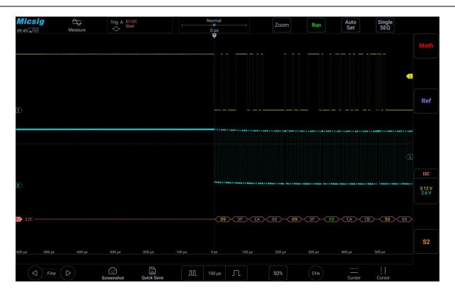
Figure 11-24 I<sup>2</sup>C Graphic Interface
