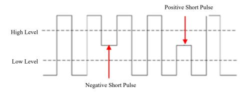
Figure 5-24 Runt Trigger
