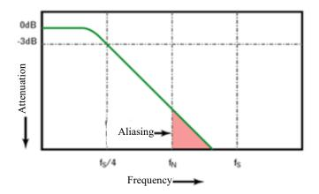
Figure 10-3 Sampling Rate and Oscilloscope Bandwidth
