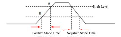
Figure 5-26 Positive/Negative Slope Time
