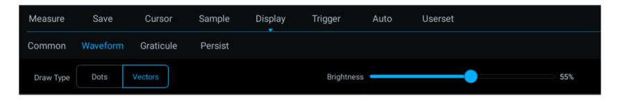
Figure 9-2 Waveform Display Menu
