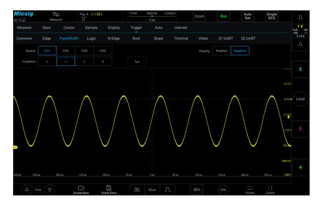
Figure 5-15 Negative Polarity Pulse Level Flip
