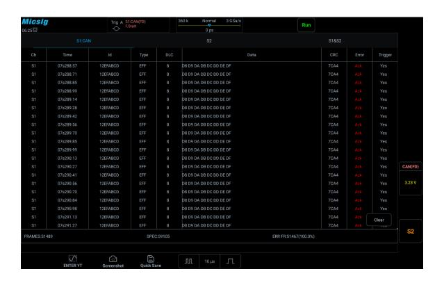
Figure 11-17 CAN bus decode in Text mode
