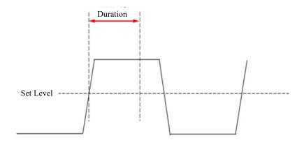
Figure 5-28 Timeout Trigger Schematics
