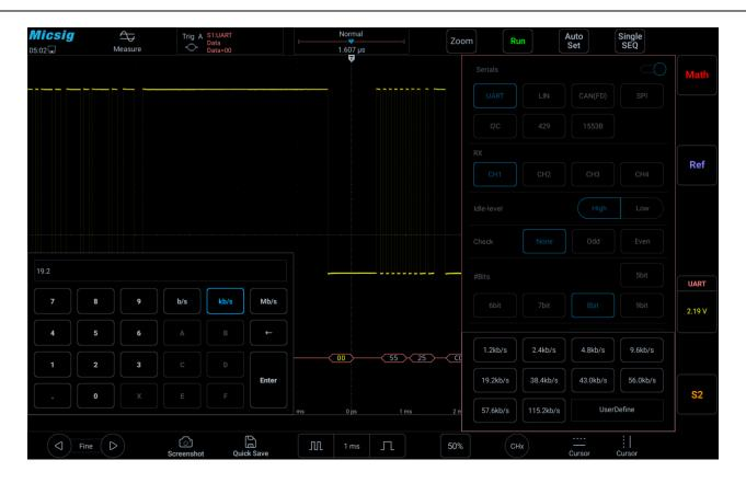
Figure 11-5 Baud Rate Default Setting
