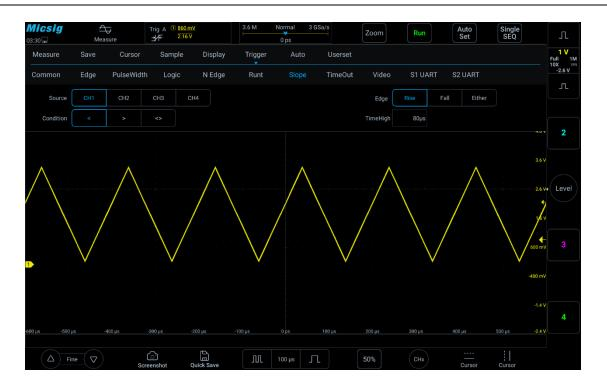
Figure 5-27 Slope Trigger Setting Menu
