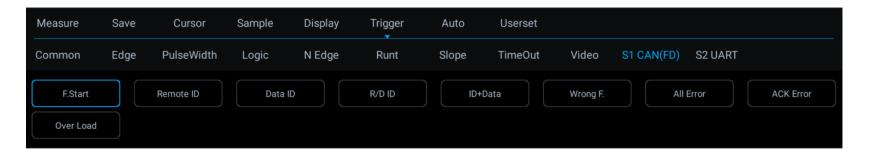
Figure 11-15 CAN FD Trigger Mode Configuration Menu
