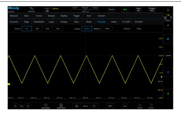
Figure 5-29 Time-out Trigger
