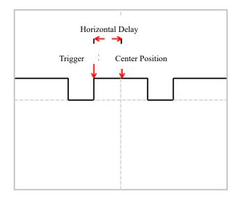
Figure 5-7 Horizontal Delay
