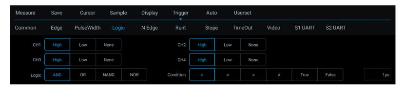
Figure 5-21 Logic Trigger Setting Menu
