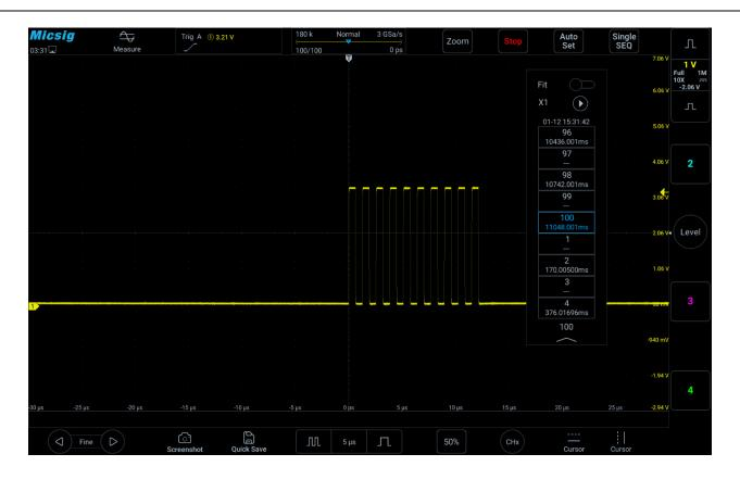
Figure 10-12 Segmented storage single frame viewing
