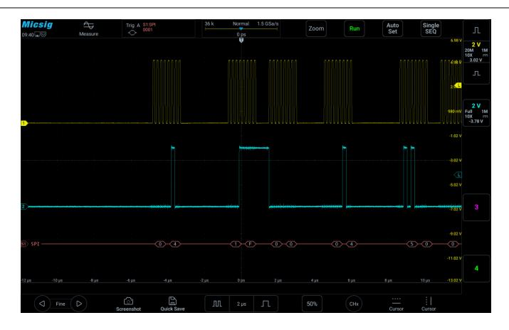
Figure 11-20 SPI bus decode interface
