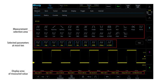
Figure 6-1 Automatic Measurement Menu
