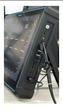
Figure 2-13 Probe Connection
