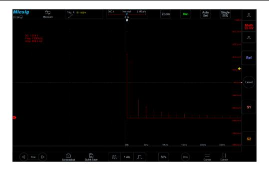
Figure 8-4 Spectrum Amplitude as V-Hz
