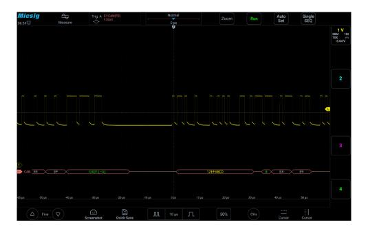
Figure 11-16 CAN bus decode interface
