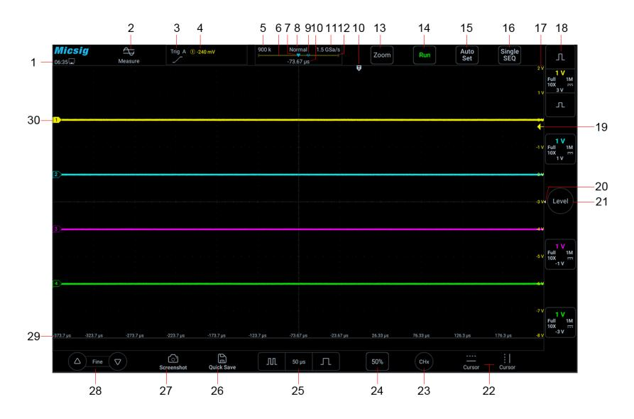
Figure 2-6 Oscilloscope Interface Display
