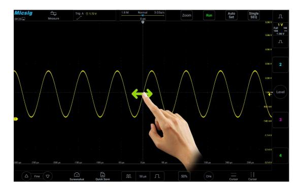
Figure 3-1 Move the Waveform Horizontally on the Screen
