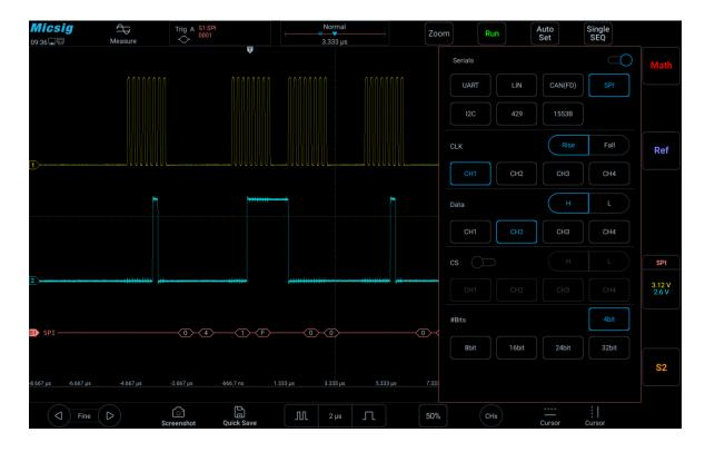
Figure 11-18 SPI Bus Configuration Menu
