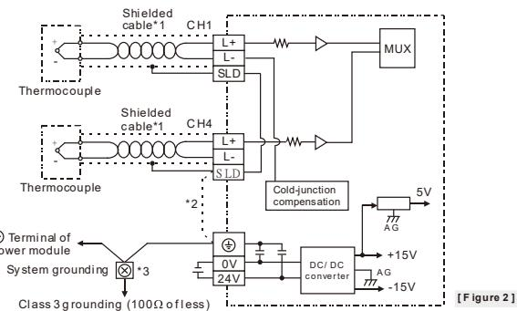
**Note1:** Use only the wires that are supplied with your thermocouple sensor. Tighten PLC terminal screws to a torque of 1.95 kg-cm (1.7 in-lbs).
