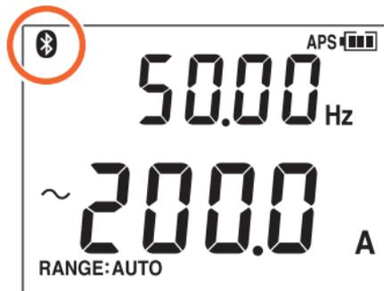
Bluetooth icon will flash when the instrument is connected to a mobile device.
