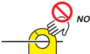
**Do not clamp around two wires.**
