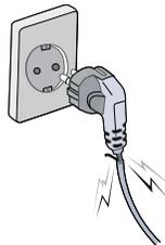
If a power plug is broken or a plug is cut or worn, do not use it.
