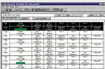
**Closed-loop calibration system for METRAHIT multimeters with METRAwin 90-F/FJ, a PC with IEEE 488 interface and a Fluke 5500A, 5520A or 5700A calibrator**
