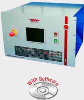
**2/3-channel microohmmeter in 19" rack for up to 100 A / 50 V for testing contact, connection and winding resistance at inductances of up to 1500 Henry in the high and medium-voltage ranges, as well as continuity testing and length measurement for cables and cable shielding (transformers, generators, motors)**
