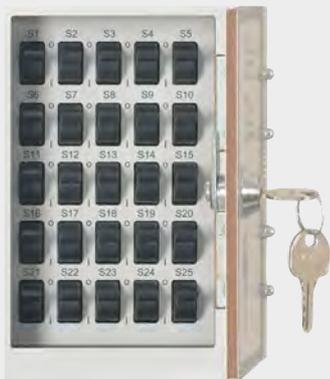
Error Simulator with 25 Error Options via Switches
