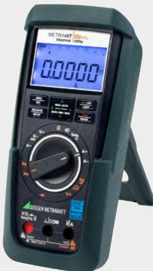
Special multimeter for connection to current transformers without fuses, in order to eliminate danger resulting from interruption of the transformer circuits (and thus measuring category 600 V CAT II)
