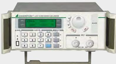
Series SSL devices (single-channel system load) are programmable electronic loads with a maximum sink power of 150 or 300 W. They're used for loading direct voltage sources with constant current, resistance or power in an adjustable fashion. Their range of applications includes testing power packs, batteries, PV modules, fuel cells etc.
