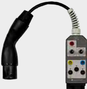
Single and 3-phase test adapter with type 2 plug for testing the effectiveness of protective measures at electric charging stations with the PROFITEST MTECH+ / MXTRA, simulation of fictitiously connected electric vehicles and current-carrying capacity of cord sets per IEC 61851-1
