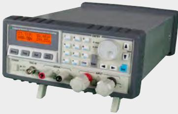
Series SPL devices (single-channel programmable load) are programmable electronic loads with outstanding dynamic control characteristics. They're used for loading direct voltage/current sources with constant current, resistance, voltage or power in an adjustable fashion. Their range of applications includes static and dynamic testing of power packs, batteries, PV modules, fuel cells, inductors etc.
