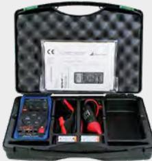
4¾ place milliohmmeter for potentially explosive atmospheres – for measuring low-value contact resistance in explosive atmospheres, e.g. at contacts inside aircraft fuel tanks (bonding test), as well as for general low-value resistance measurements inside and outside of potentially explosive atmospheres, for example on aircraft outer skins (lightning protection and wick test)
