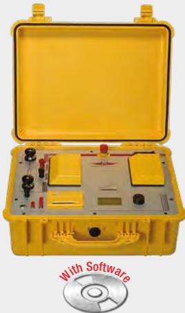
Microohmmeter for up to 200 A for testing contact and connection resistance
