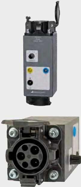
Single-phase test adapter with type 1 plug for testing the effectiveness of protective measures at electric charging stations with the PROFITEST MTECH+ / MXTRA, simulation of fictitiously connected electric vehicles and current-carrying capacity of cord sets per IEC 61851-1
