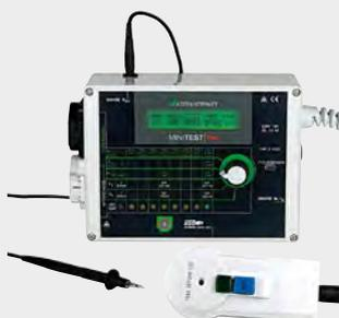
Test instrument for **DIN VDE 0701-0702**, for testing and measurement of repaired or modified devices
