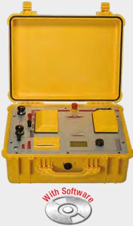
**2/3-channel microohmmeter for up to 50 A / 50 V for testing contact, connection and winding resistance at inductances of up to 1500 Henry in the high and medium-voltage ranges, as well as continuity testing and length measurement for cables and cable shielding (transformers, generators, motors)**
