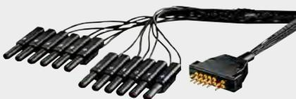
Adapter cable for SECUTEST, SECULIFE ST for adapting the 2 mm connector sockets at the SECUTEST / SECULIFE ST to 4 mm sockets and plugs, 1.5 m long with 12 cables, each with 4 mm plug
