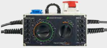
**Adapter for standards-compliant testing of type S and K PRCDs by simulating faults and manufacturer specifications.**
