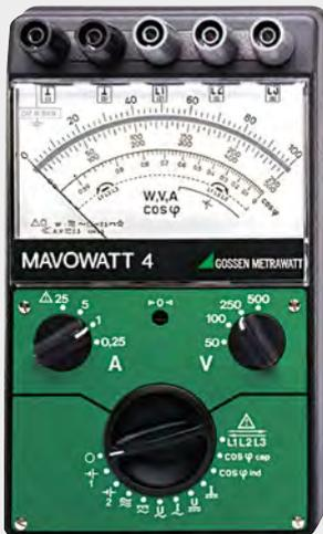
The multiple power meter for direct measurement of DC power, as well as RMS power measurement for single-phase alternating current and balanced load three-wire, three-phase current.
