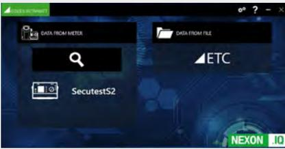
NEXONIQ is an optional module for IZYTRONIQ. NEXONIQ makes it possible to read out the test instrument memory and simultaneously convert it to the IZYTRONIQ format. Additionally, it permits data conversion of existing ETC files for transfer to IZYTRONIQ.
