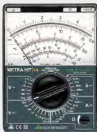
**Compact, basic analog multimeter for training and hobby, and for electrical applications**
