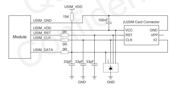
Figure 12: Reference Circuit of (U)SIM Interface with a 6-Pin (U)SIM Card Connector
