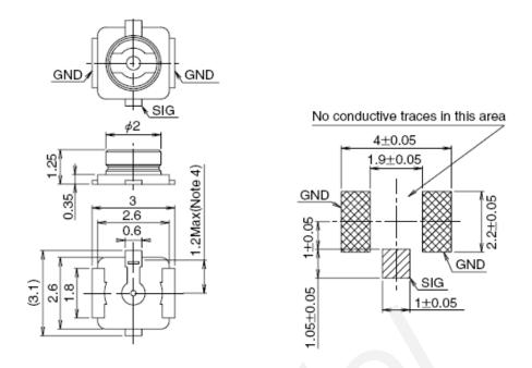
Figure 26: Dimensions of the UF.L-R-SMT Connector (Unit: mm)
