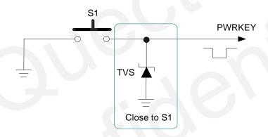
Figure 5: Turn on the Module Using Keystroke
