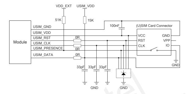
Figure 11: Reference Circuit of (U)SIM Interface with an 8-Pin (U)SIM Card Connector
