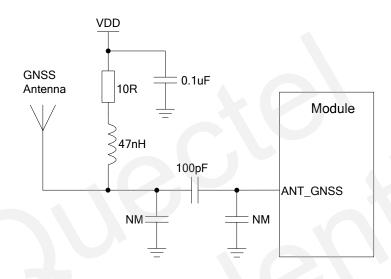
Figure 25: Reference Circuit of GNSS Antenna Interface
