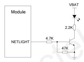
Figure 17: Reference Circuit of the Network Status Indicator
