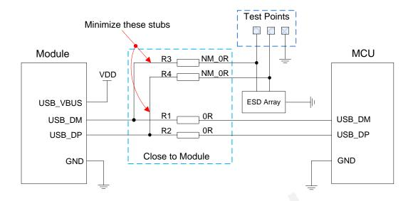
Figure 13: Reference Circuit of USB Application
