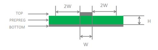
Figure 21: Microstrip Line Design on a 2-layer PCB
