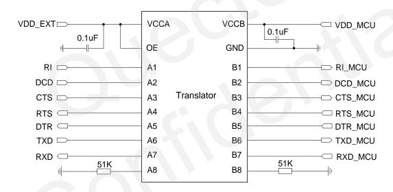
Figure 14: Reference Circuit with Translator Chip
