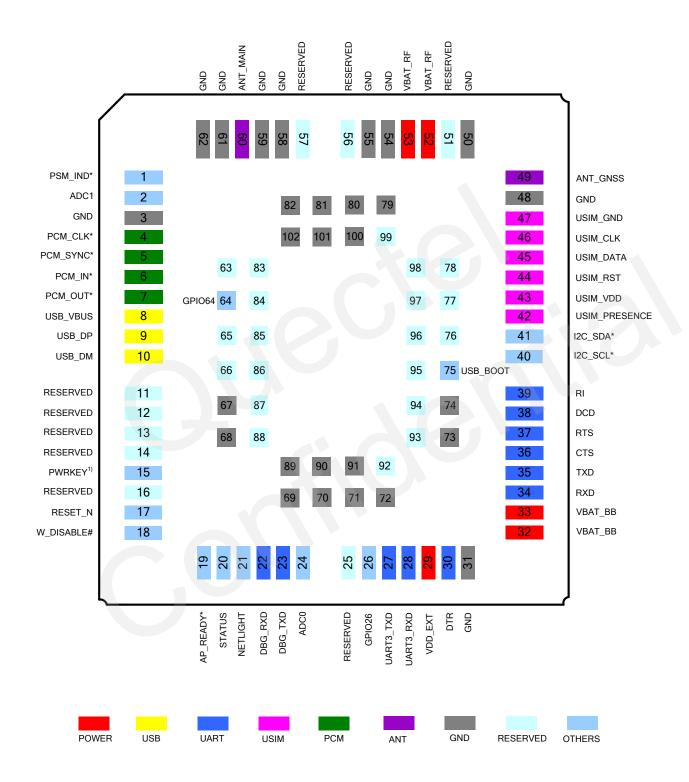
Figure 2: Pin Assignment (Top View)
