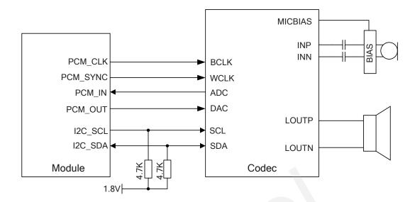
Figure 16: Reference Circuit of PCM Application with Audio Codec
