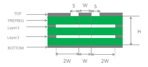
Figure 24: Coplanar Waveguide Line Design on a 4-layer PCB (Layer 4 as Reference Ground)
