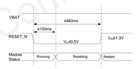
Figure 10: Timing of Resetting Module
