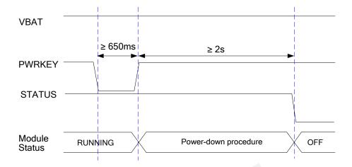
Figure 7: Timing of Turning off Module
