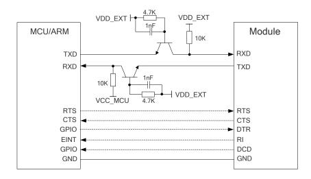
Figure 15: Reference Circuit with Transistor Circuit
