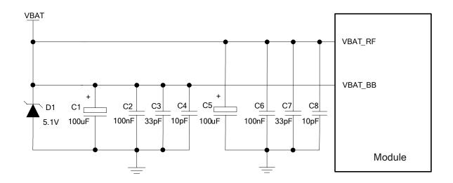
Figure 3: Star Structure of the Power Supply
