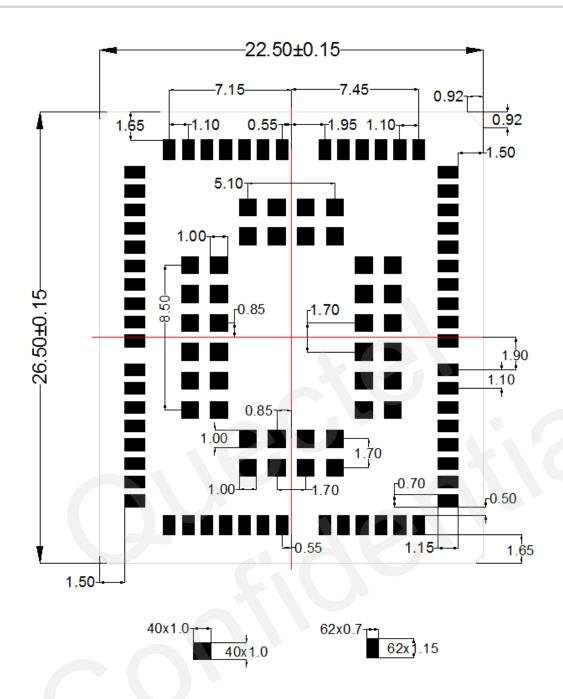
Figure 30: Module Bottom Dimensions (Bottom View)
