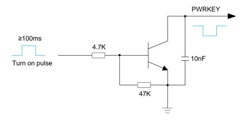
Figure 4: Turn on the Module Using Driving Circuit
