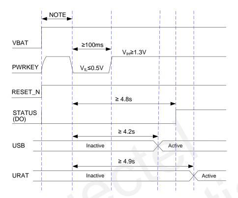
Figure 6: Timing of Turning on Module
