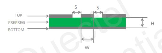
Figure 22: Coplanar Waveguide Line Design on a 2-layer PCB
