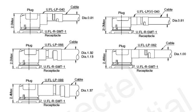
Figure 28: Space Factor of Mated Connector (Unit: mm)
