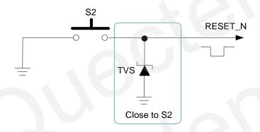
Figure 9: Reference Circuit of RESET\_N by Using Button
