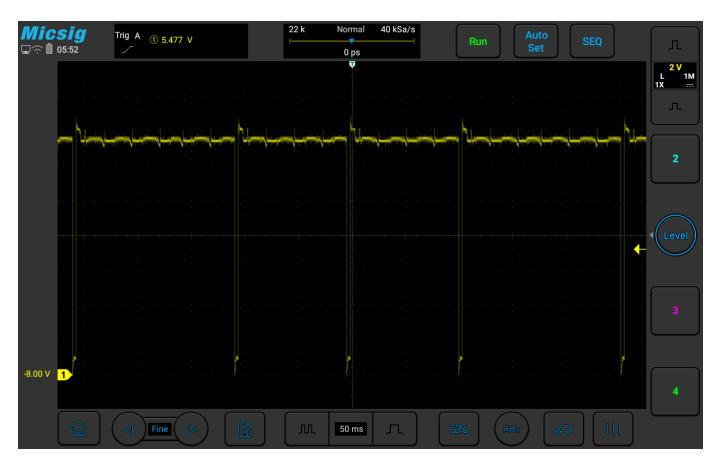
Figure 3-27 Audi A6 Carbon canister solenoid valve signal
