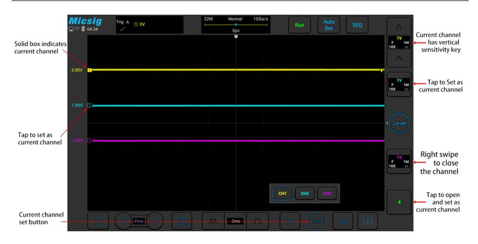
Figure 5-4 Channel Open, Close and Switching
