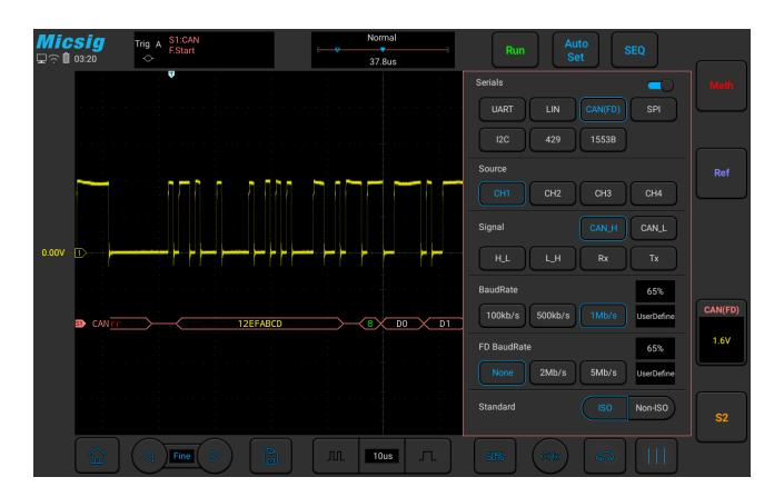
Figure 12-14 CAN Bus Configuration Menu
