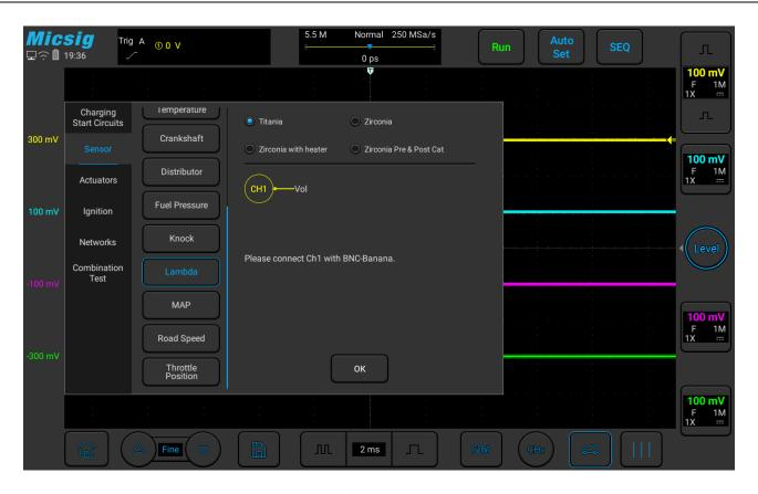
Figure 3-20 Lambda (oxygen sensor) test
