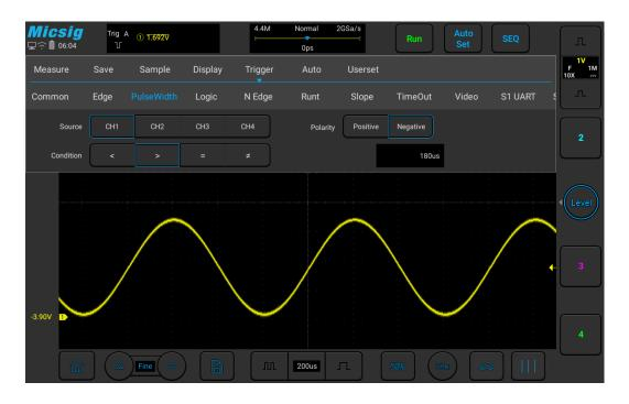
Figure 6-15 Negative Polarity Pulse Level Flip
