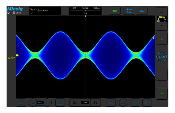
Figure 10-5 Color Temperature Open Mode
