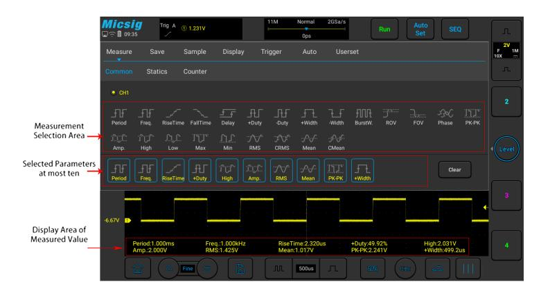
Figure 7-1 Automatic Measurement Menu
