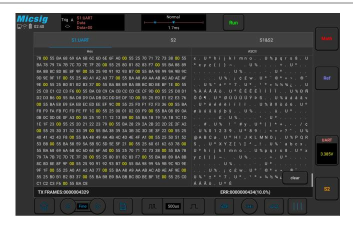
Figure 12-2 Bus Decode Text Mode
