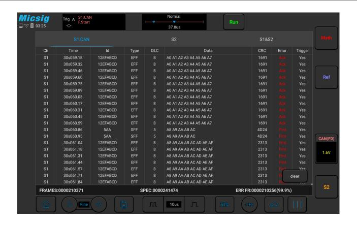
Figure 12-17 CAN Text Interface
