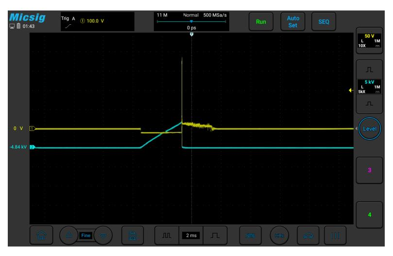
Figure 3-44 BMW 5 Series N20 Primary + Secondary ignition signal
