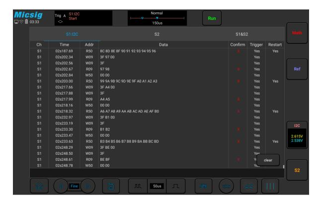
Figure 12-25 I2C Text Interface
