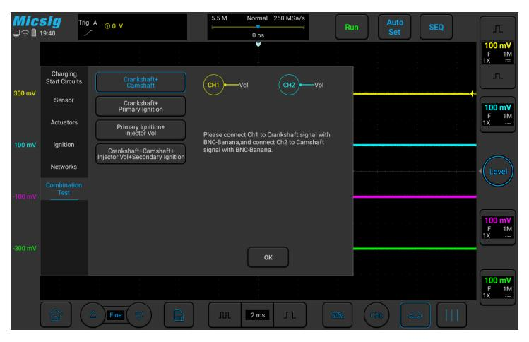
Figure 3-50 Crankshaft + Camshaft Combination Test
