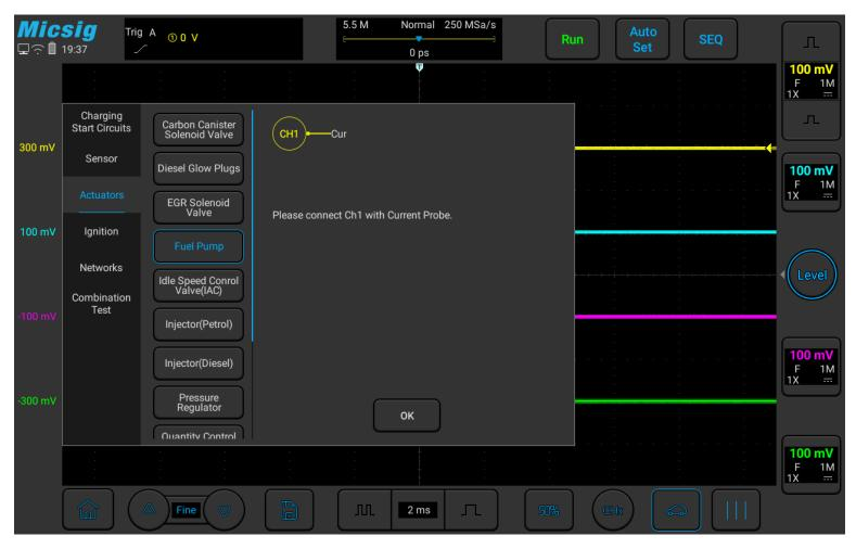
Figure 3-30 Electronic fuel pump test
