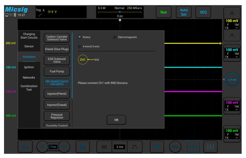
Figure 3-31 Idle speed control valve test
