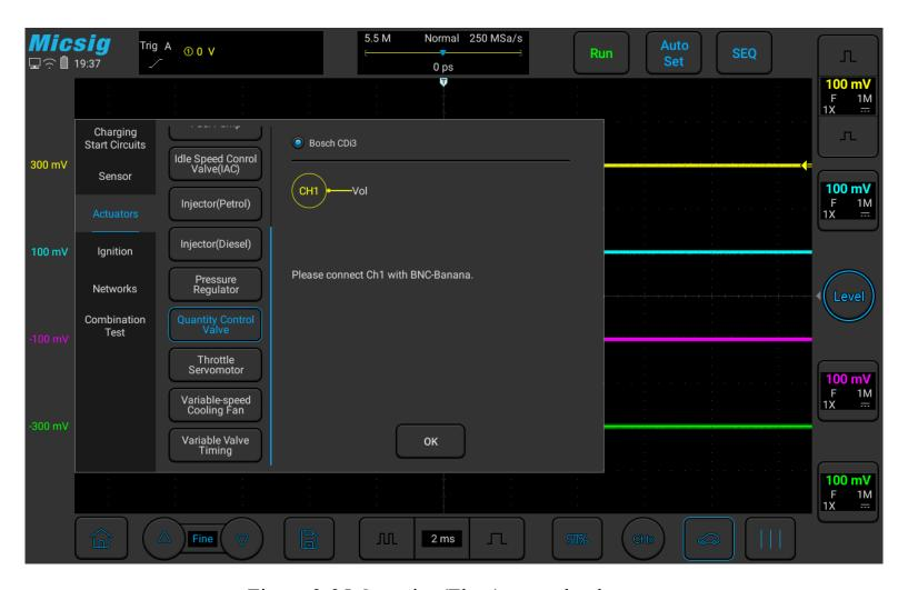
Figure 3-35 Quantity (Flow) control valve test
