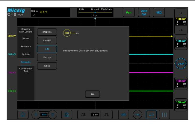
Figure 3-46 Lin bus test
