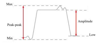
Figure 7-7 Voltage Measurement
