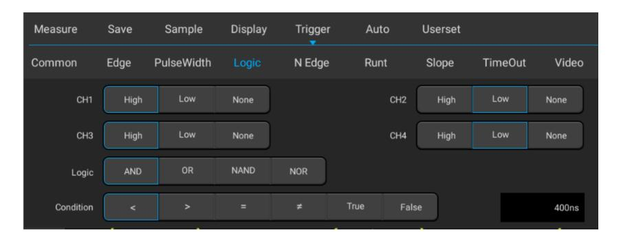
Figure 6-21 Logic Trigger Setting Menu
