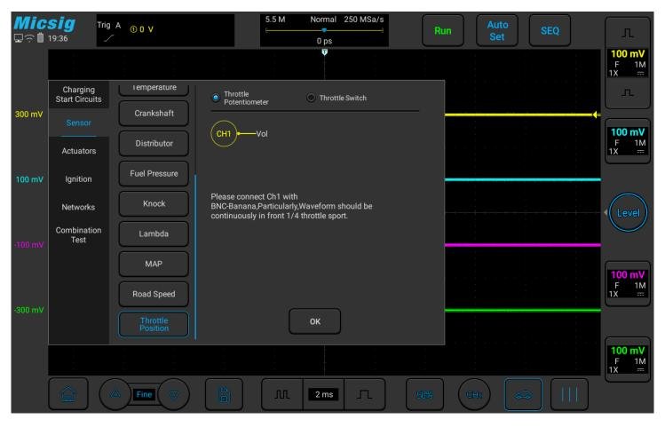
Figure 3-24 Throttle Position Sensor test
