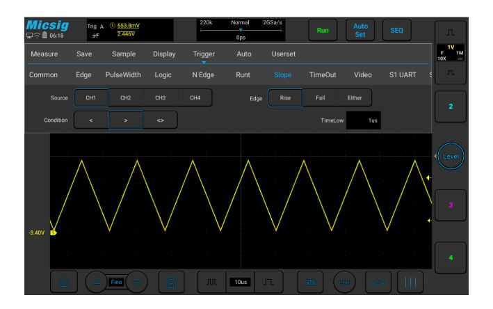
Figure 6-27 Slope Trigger Setting Menu
