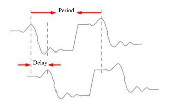
Figure 7-6 Phase Measurement Schematics
