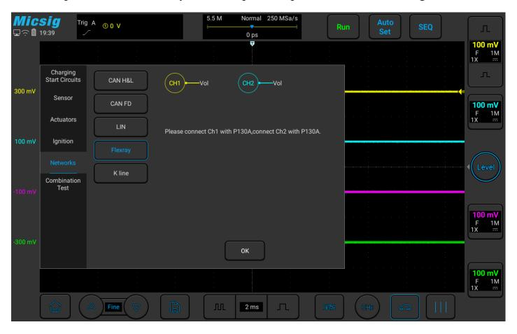
Figure 3-48: FlexRay bus test
