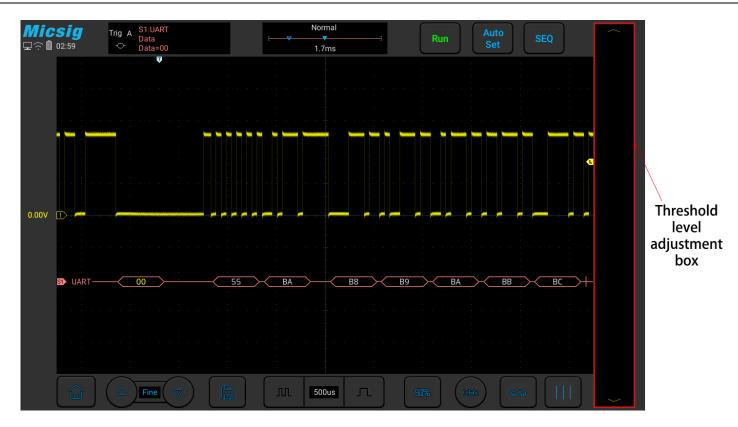
Figure 12-7 UART Decode Level Adjustment
