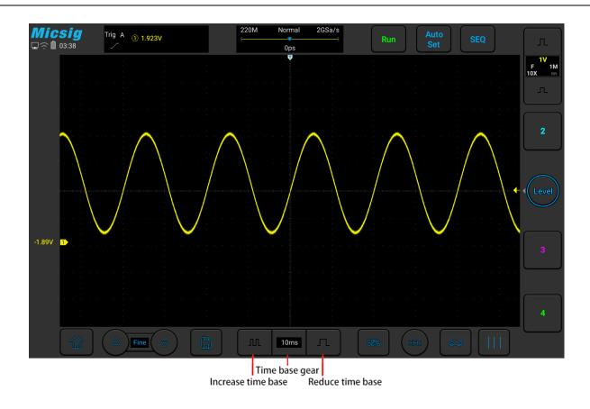
Figure 4-3 Adjust the Horizontal Time Base
