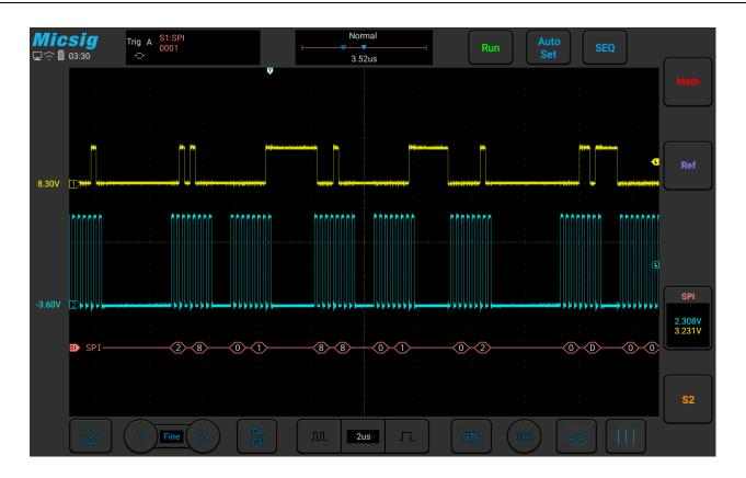
Figure 12-20 SPI Graphic Interface
