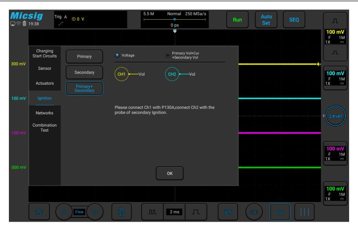
Figure 3-43: Primary + Scondary ignition test
