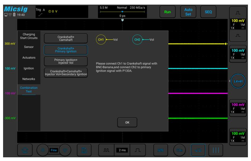
Figure 3-51 Crankshaft + Primary ignition test
