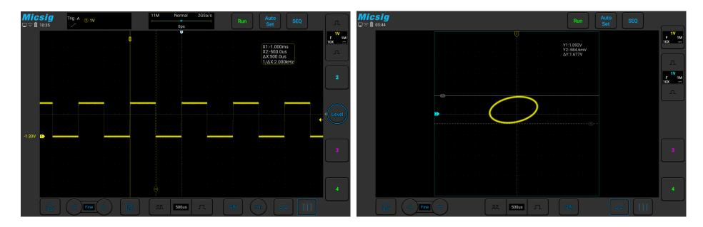
Figure 7-13 Cursor Measurement Pulse Width
