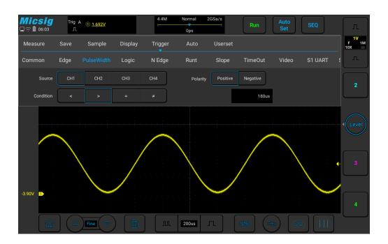
Figure 6-14 Pulse Width Trigger Setting Menu
