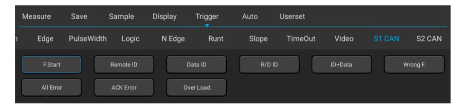
Figure 12-15 CAN Trigger Mode Configuration Menu
