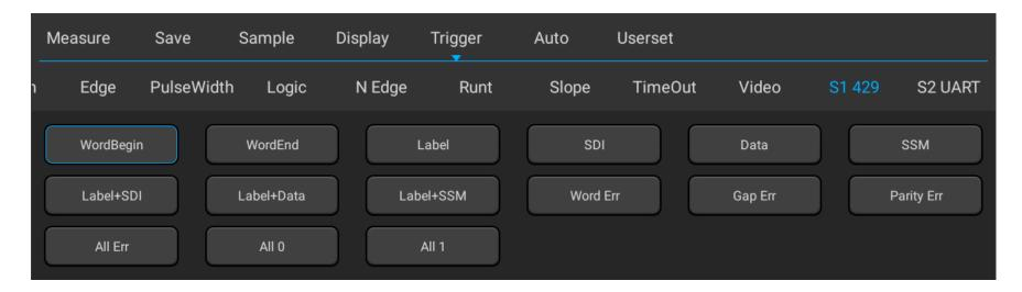
Figure 12-27 ARINC429 Trigger Mode Configuration Menu
