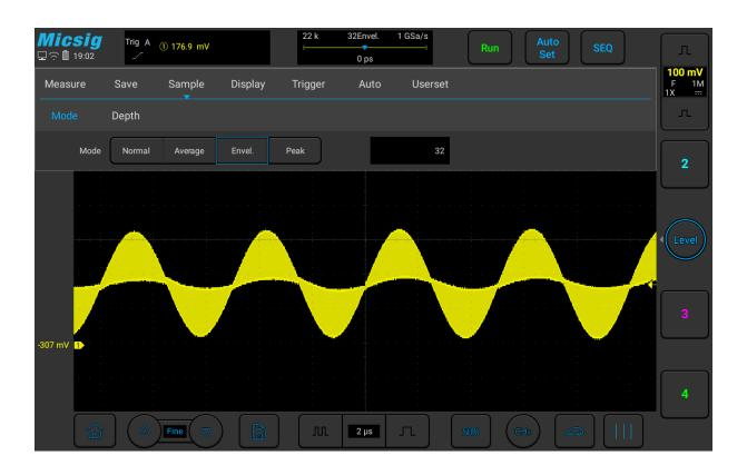
Figure 11-8 AM Signal in Envelope Sampling Mode (32)
