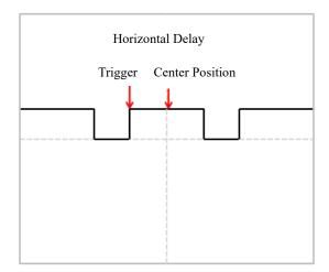
Figure 6-7 Horizontal Delay
