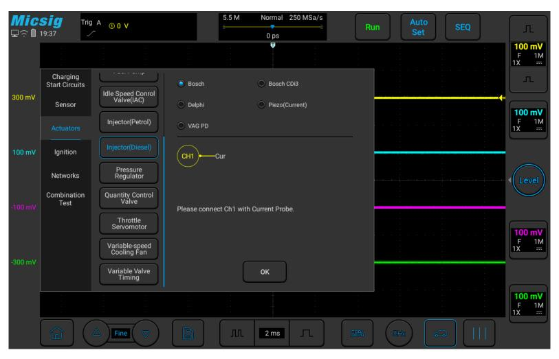
Figure 3-33 injector (diesel engine) test
