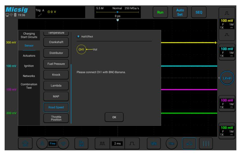
Figure 3-23 Vehicle speed sensor test
