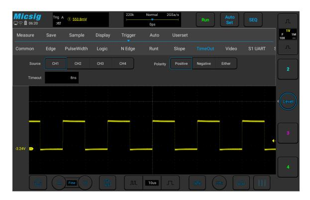
Figure 6-29 Time-out Trigger
