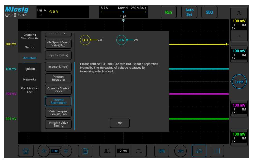
Figure 3-36 Throttle servo motor test
