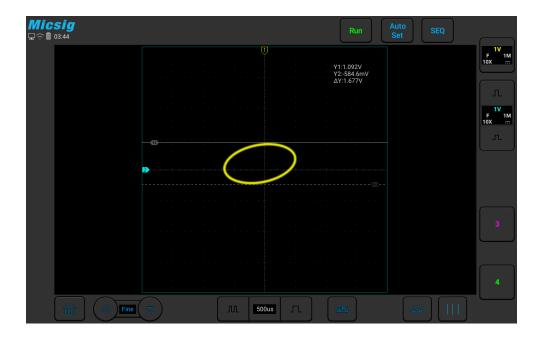
Figure 4-10 Phase Difference Measurement and Using the Cursor
