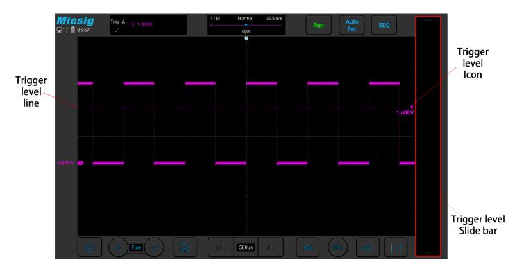
Figure 6-8 Trigger Level
