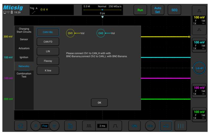
Figure 3-45 CAN BUS Test
