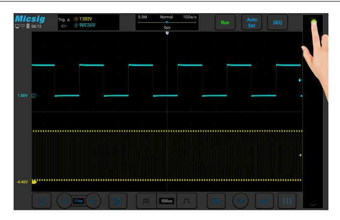
Figure 6-22 Trigger Level Adjustment
