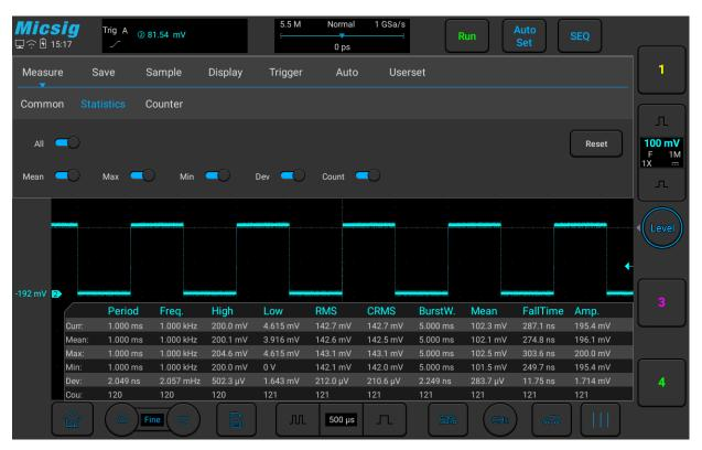
Figure 7-8 Frequency Meter Measurement Menu Open
