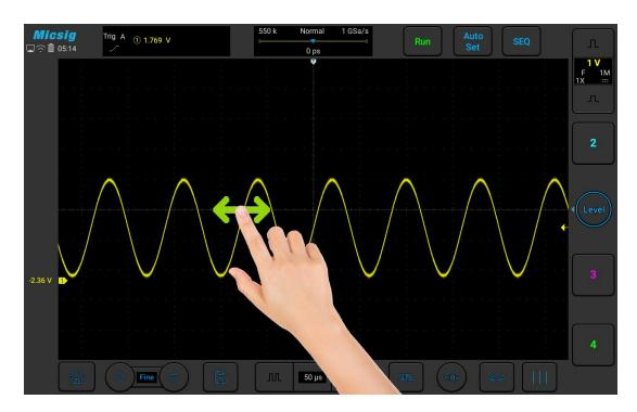
Figure 4-2 Move the Waveform Horizontally on the Screen
