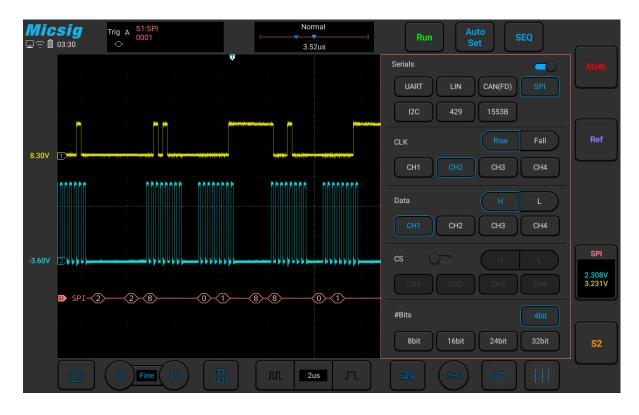
Figure 12-18 SPI Bus Configuration Menu
