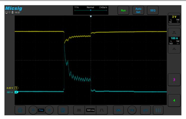
Figure 3-7 Starting voltage and current
