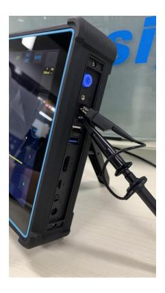
Figure 2-13 Probe Connection
