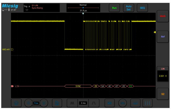
Figure 3-47 Audi A6 LIN bus measurement
