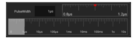
Figure 6-20 Pulse Width Time Adjustment Interface
