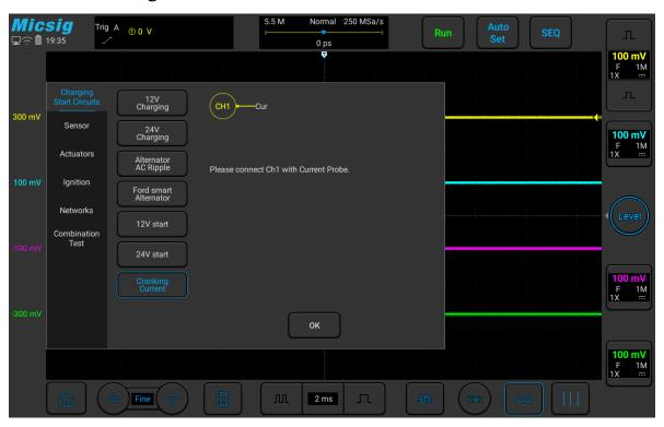
Figure 3-9 Cranking Current
