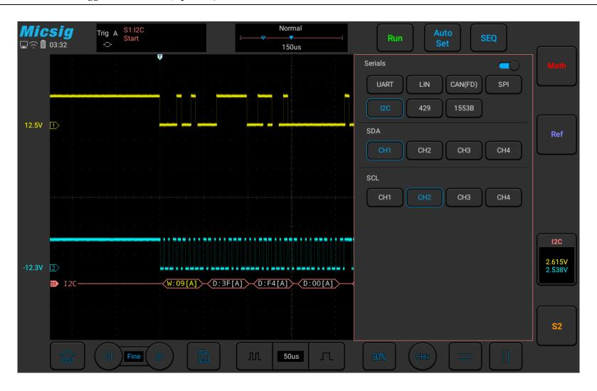
Figure 12-22 I2C Bus Configuration Menu
