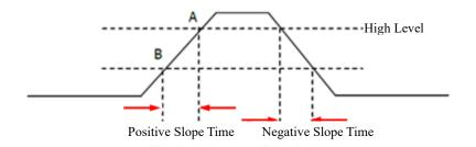
Figure 6-26 Positive/Negative Slope Time
