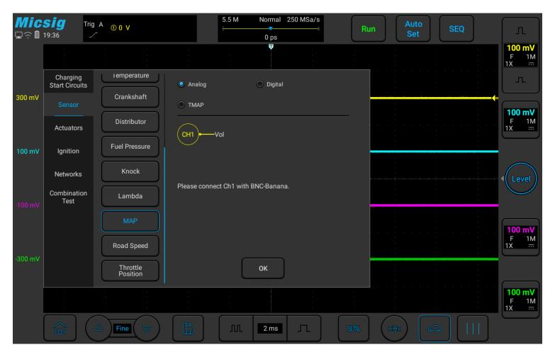
Figure 3-22 MAP (intake pressure sensor)
