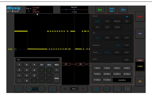
Figure 12-5 Baud Rate Default Setting
