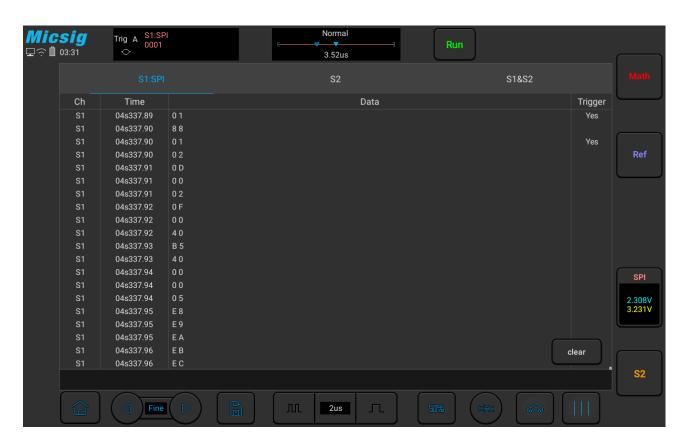
Figure 12-21 SPI Text Interface
