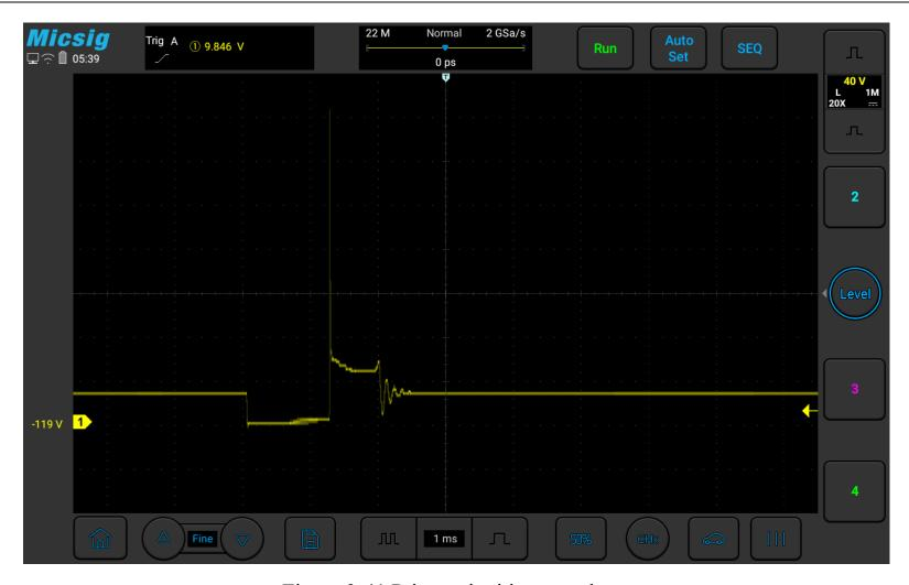
Figure 3-41 Primary ignition actual test
