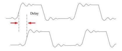
Figure 7-5 Delay Measurement Schematics
