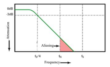
Figure 11-3 Sampling Rate and Oscilloscope Bandwidth
