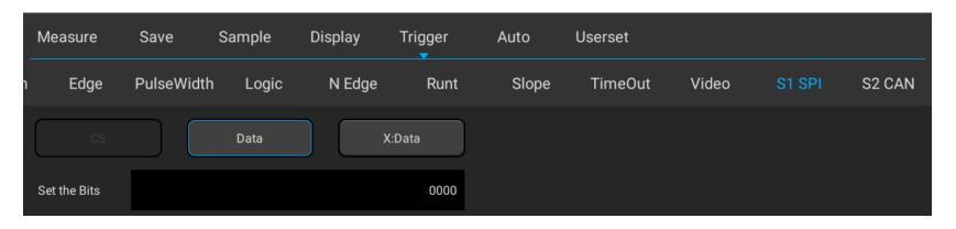
Figure 12-19 SPI Trigger Mode Configuration Menu
