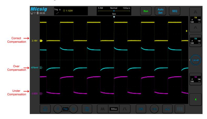
Figure 2-14 Probe Compensation
