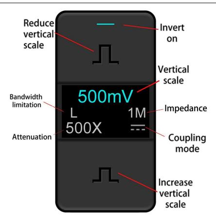
Figure 5-3 Channel Display Interface
