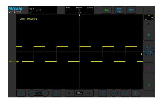
Figure 7-10 Frequency Meter Measurement
