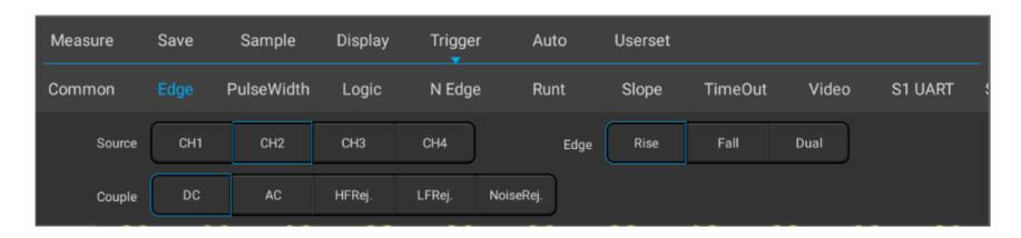
Figure 6-12 Edge Trigger Setting Menu
