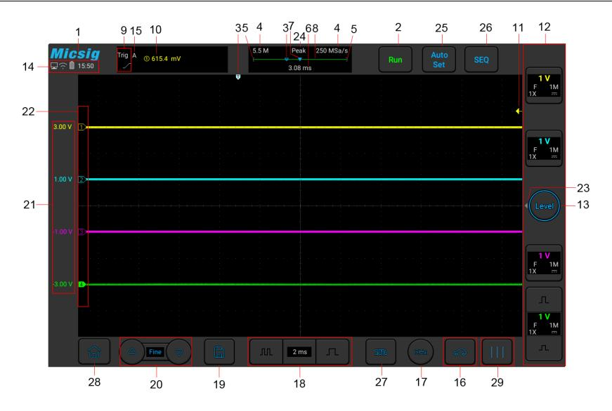
Figure 2-6 Oscilloscope Interface Display
