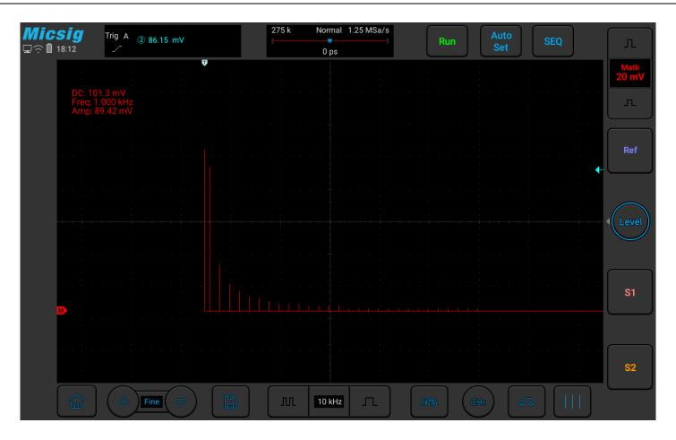
Figure 9-4 Spectrum Amplitude as V-Hz
