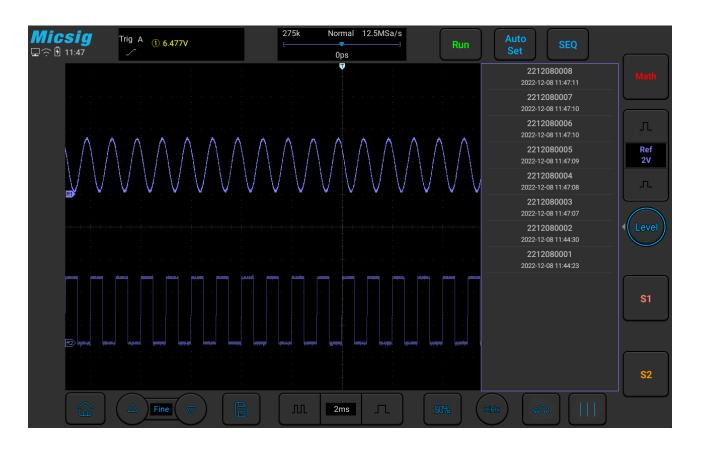
Figure 9-7 Restore Reference Waveform
